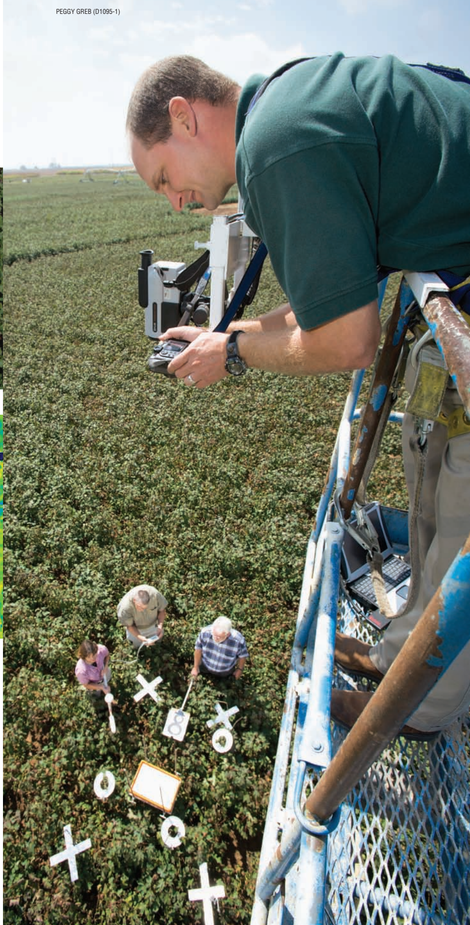
Technician Brice Ruthardt takes vertical images in the infrared and ordinary spectrums of cotton under water stress. Agricultural engineers Susan O'Shaughnessy (left) and Terry Howell (center) are taking multispectral measurements while soil scientist Steve Evett holds a reference target.
