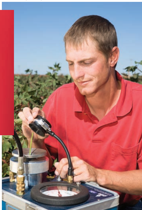
Using the pressure chamber technique (an industry standard), technician Chad Ford measures leaf water potential to determine water stress status of cotton plants. The measurements verify water stress at different crop canopy temperatures.
