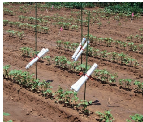
Wireless infrared thermometers continuously measure plant temperature as part of the BIOTIC irrigation scheduling method.
