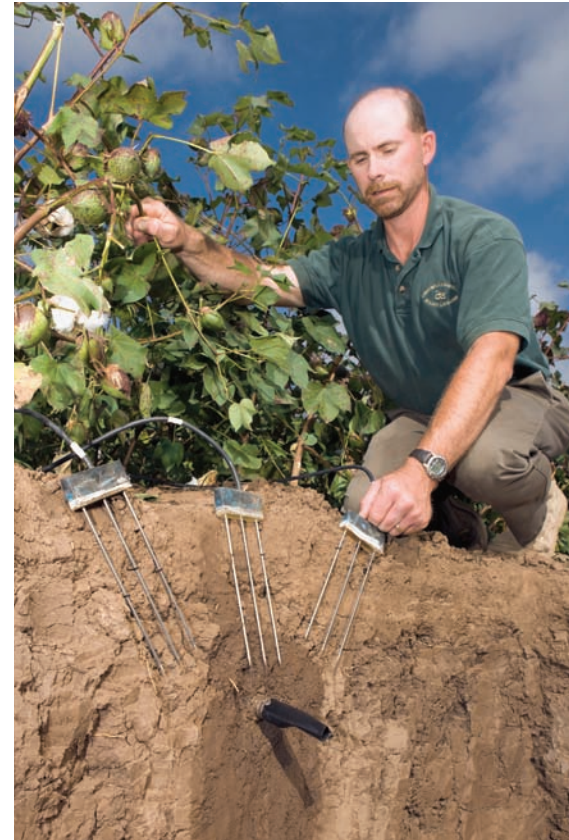
Paul Colaizzi, agricultural engineer, demonstrates the soil-wetting pattern of subsurface drip irrigation in a cottonfield and measurement of volumetric soil water content using time-domain reflectometry probes.
