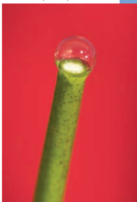
Sap bubble on the cut end of a cotton stem after leaf water potential was measured using the pressure chamber.
