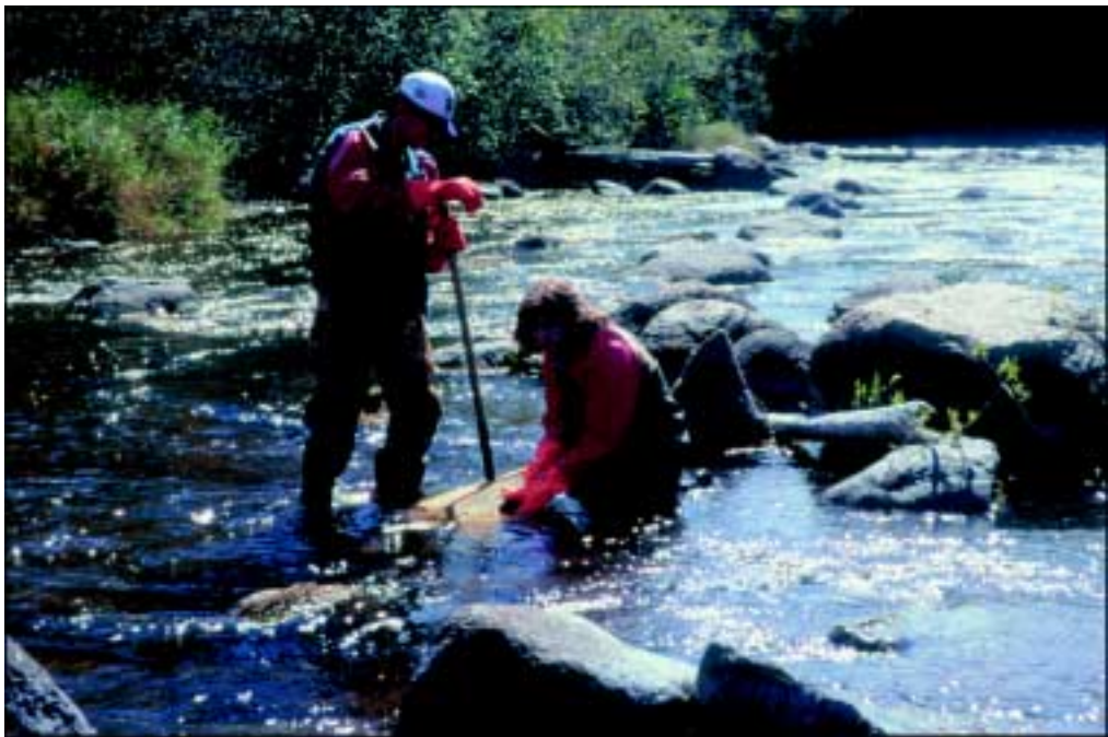
Figure 4. Invertebrate community sampling method using a modified Surber net, Wolf River near Langlade biological site.
