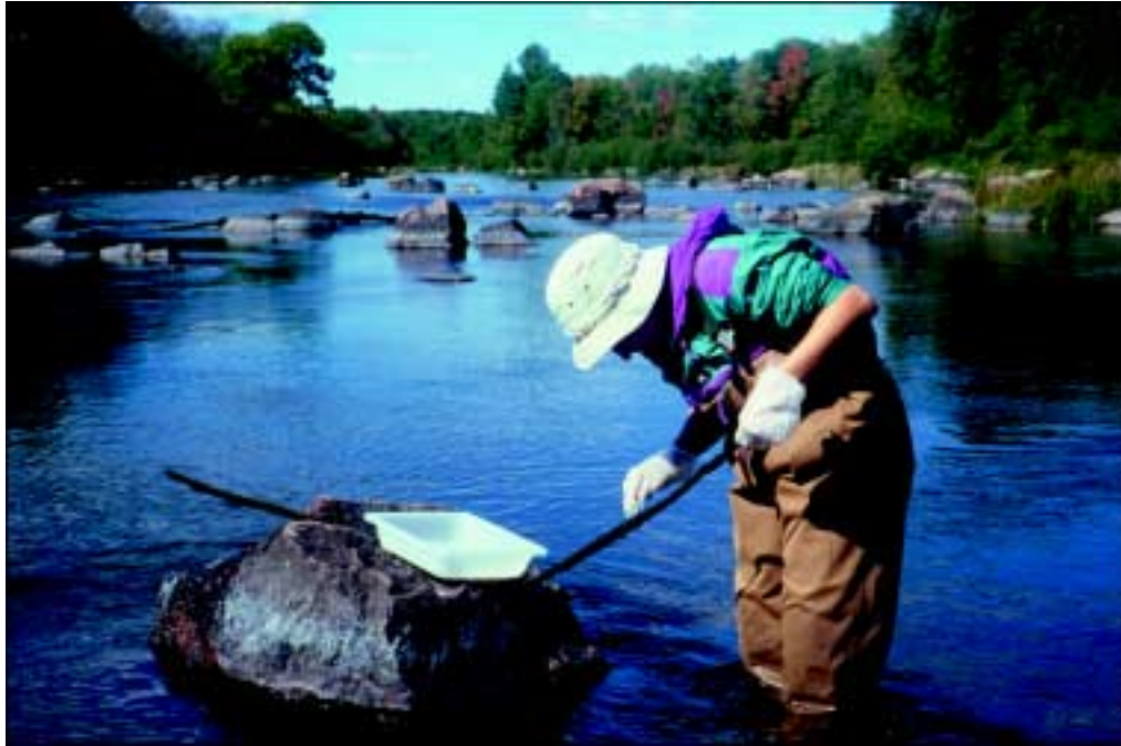
Figure 3. Method for collecting caddisfly larvae from woody debris and rocks for trace-element analysis.
