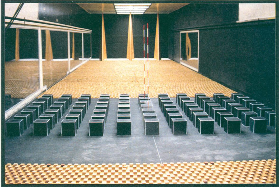
Figure 10. The three-dimensional building array as seen from the downstream end of the FMF wind tunnel.
