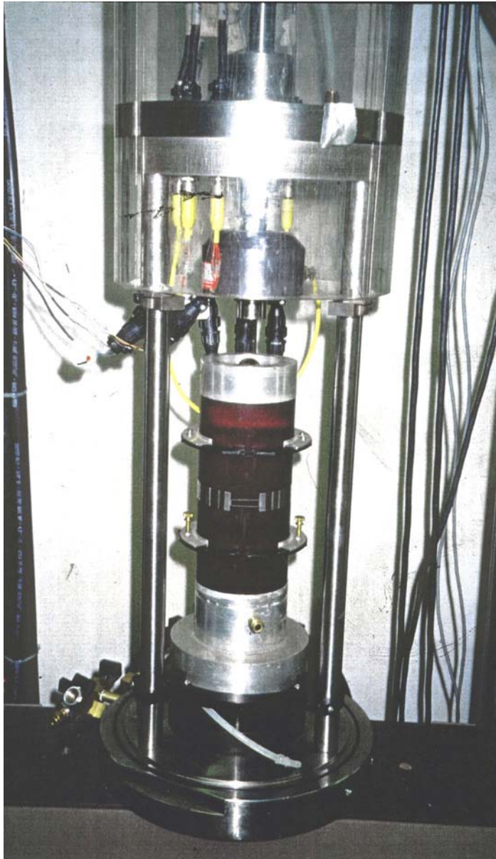
Figure 5-16. Triaxial cell set-up for resilient modulus test.
