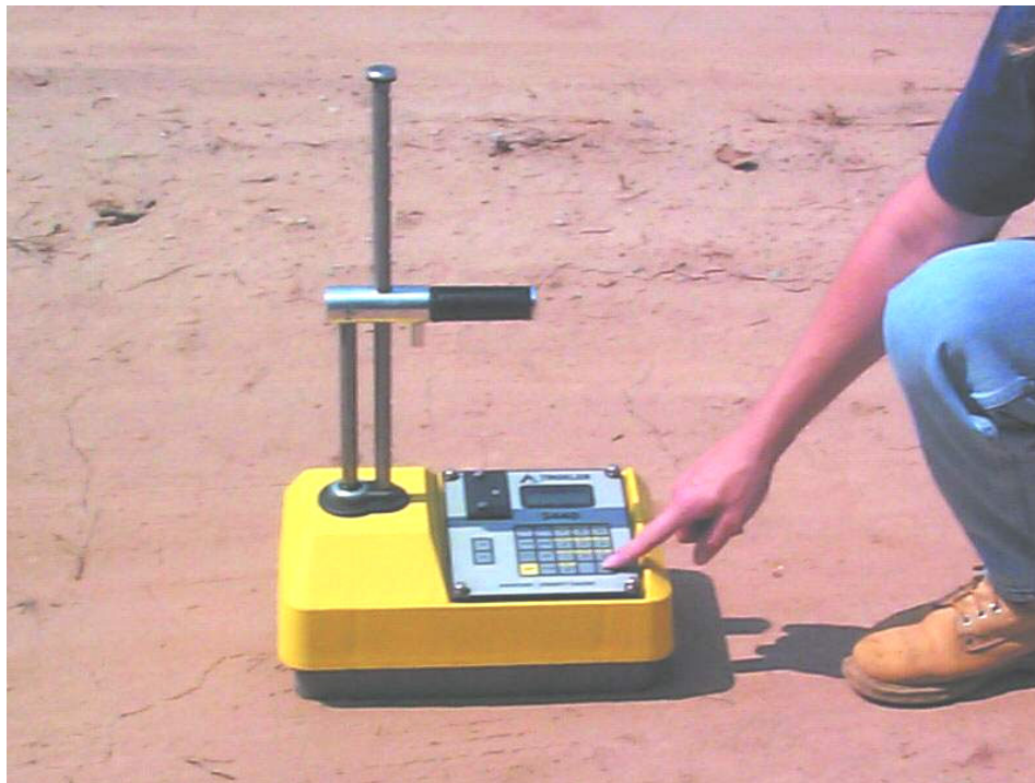
Figure 8-1. Nuclear densometer ( photo courtesy of Troxler ).
