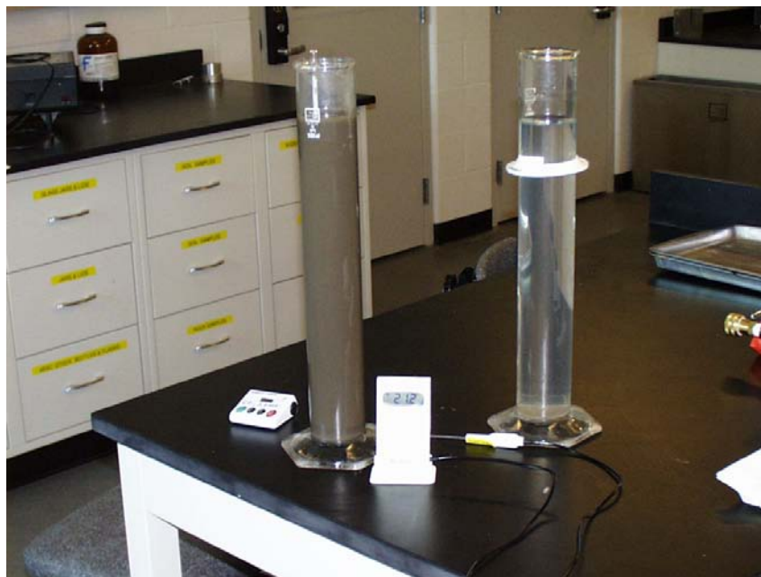
Figure 5-6. Soil hydrometer apparatus ( http://www.ce.siu.edu/ ).
