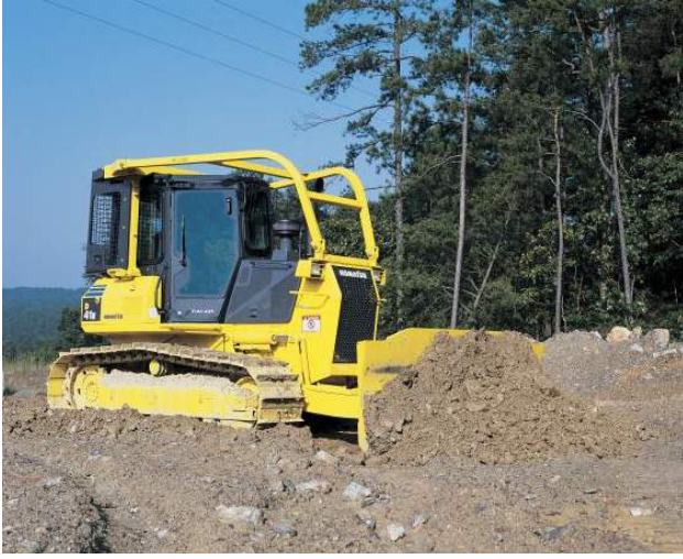
Figure 8-8. Bulldozer ( photo courtesy of Komatsu ).
