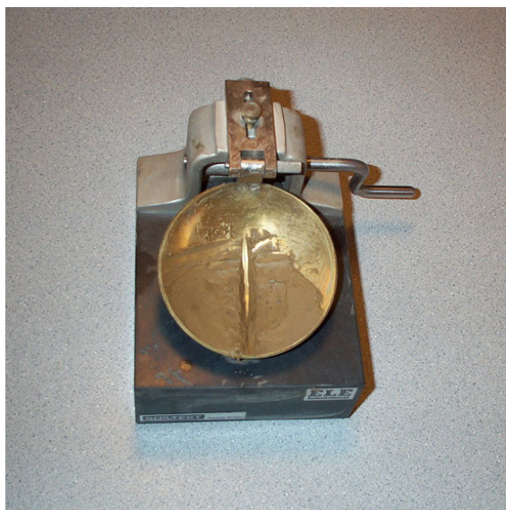
Figure 5-9. Liquid limit test device.
