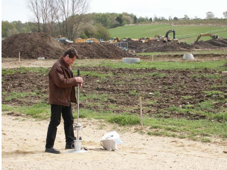
Figure 8-3. Lightweight deflectometer ( photo courtesy of Dynatest ).
