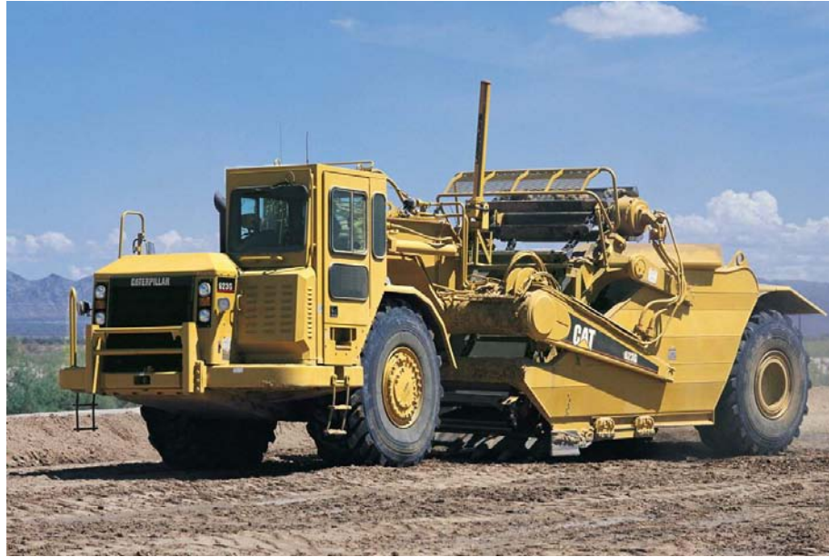
Figure 8-5. Self-loading scraper ( photo courtesy of Caterpillar ).
