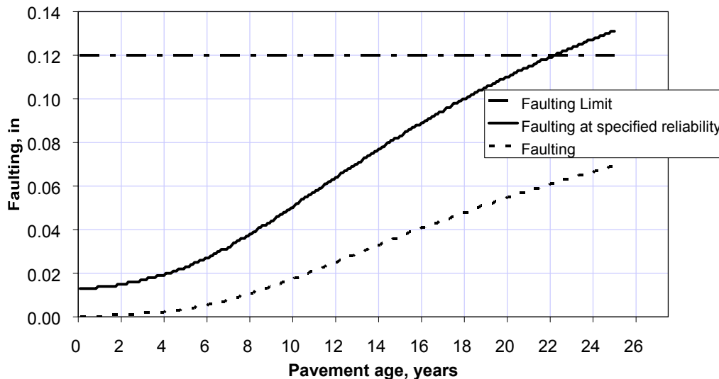
Figure 6-4. Predicted faulting performance for soft subgrade scenario.
