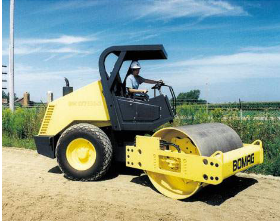
Figure 8-12. Smooth drum roller (photo courtesy of Bomag).
