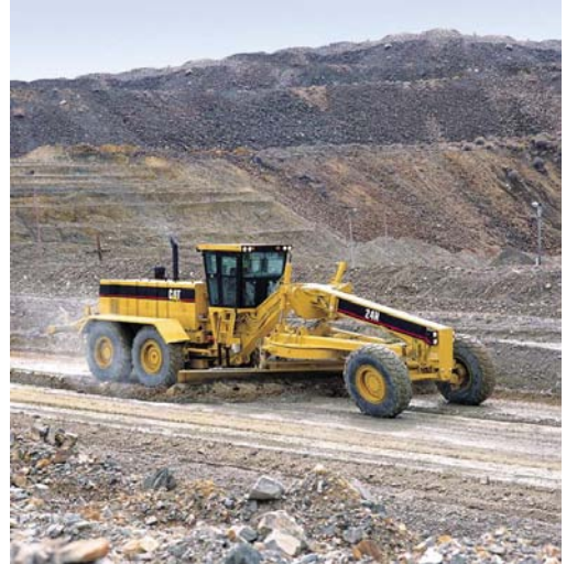
Figure 8-9. Motor grader ( photo courtesy of Caterpillar )
