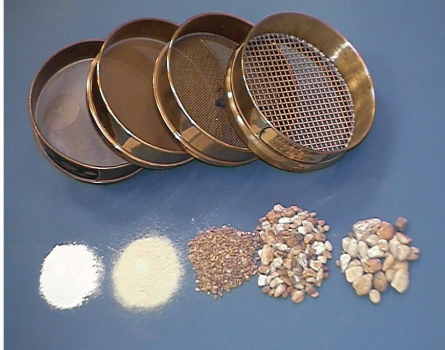
Figure 5-5. Laboratory sieves for mechanical analysis of grain size distribution. Shown (right to left) are sieve Nos. 3/8-in. (9.5-mm), No. 10 (2.0-mm), No. 40 (250- \mu\text{m} ) and No. 200 (750- \mu\text{m} ) and example soil particle sizes including (right to left): medium gravel, fine gravel, medium-coarse sand, silt, and dry clay (kaolin).
