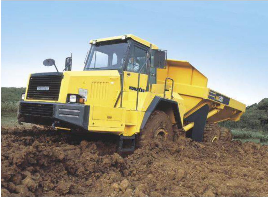
Figure 8-7. Articulated dump truck ( photo courtesy of Komatsu ).
