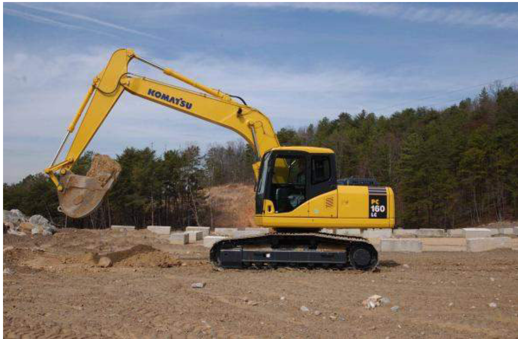
Figure 8-6. Track-mounted excavator ( photo courtesy of Komatsu ).
