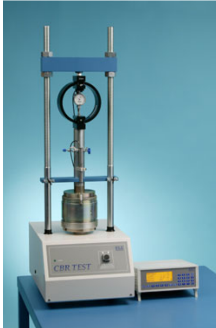
Figure 5-12. California Bearing Ratio test device ( http://www.ele.com/geot/cali.htm ).
