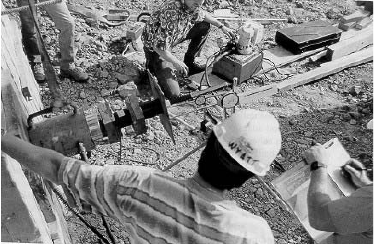
Figure 8.1: Soil Nail Load Testing Setup.
