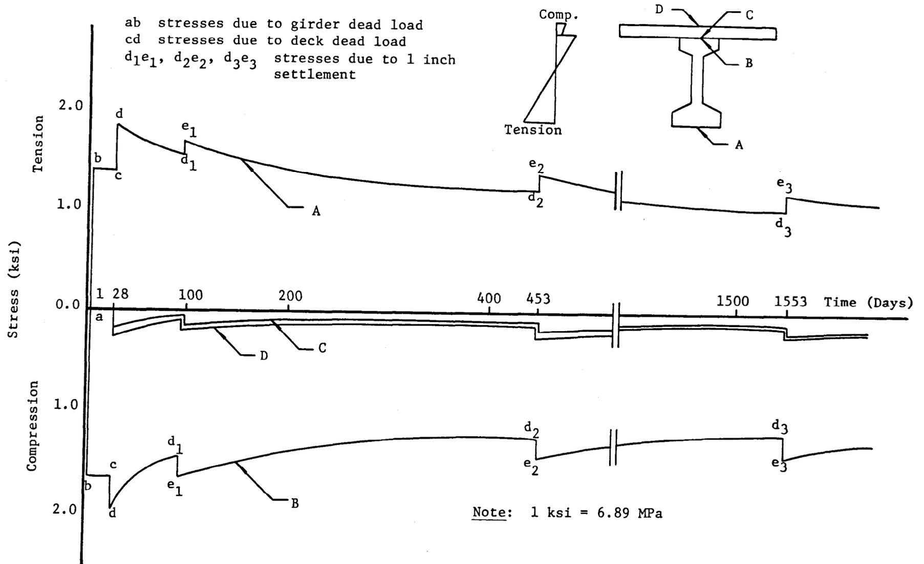
Figure 29 - Time-Dependent Variation of Stresses at Midspan for Two-Span Continuous Concrete Bridge with 100 Foot Spans - Gradual Settlement of Center Support
