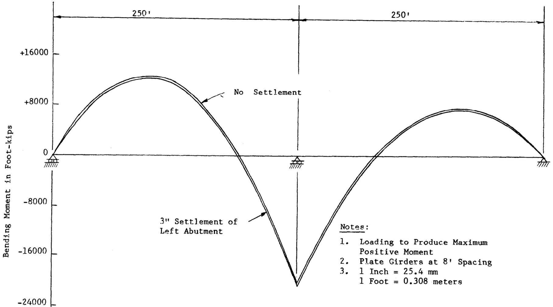
Figure 44. Typical Moment Diagram for Two-Span Continuous Bridge With 250 Foot Spans, Loaded With Dead Load, Live Load and Settlement of Left Abutment
