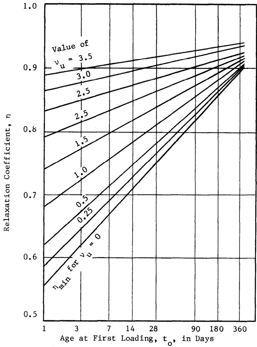
Figure 25 - Relaxation Coefficient,  $\eta$ , as a Function of the Age at First Loading,  $t_0$ , for Different Values of Ultimate Creep Coefficient,  $v_u$  (23)
