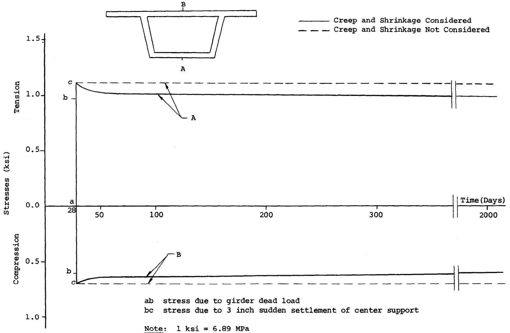
Figure 34 - Time-Dependent Stresses at Midspan for Two-Span Concrete Box Girder Bridge with 200 Foot Spans - Sudden Settlement of Center Support
