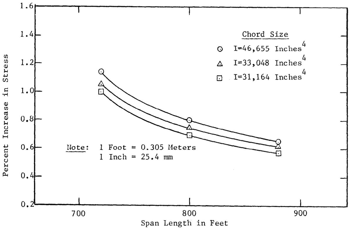
Figure 15 - Theoretical Percent Increase in Stress at Quarter Point of Two-Span Continuous Non-Parallel Chord Trusses Caused by 3 Inch Pier Settlement
