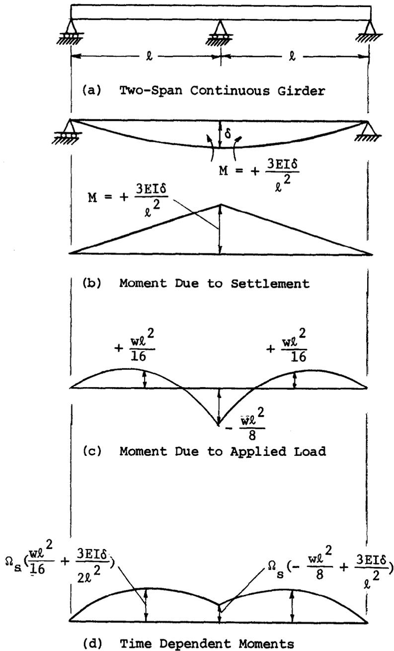
Figure 38 - Bending Moments Due to Applied Load and Settlement for Two-Span Continuous Girder
