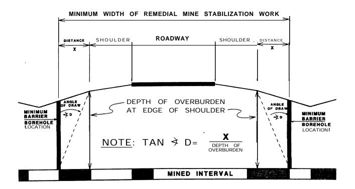
$\frac{\text{MINIMUM BARRIER}}{\text{BOREHOLE DISTANCE}} = \text{DISTANCE X} = \left[ \begin{pmatrix} \text{Depth of overburden} \\ \text{AT EDGE OF} \end{pmatrix} (TAN \Rightarrow D) \\ \frac{\text{FROM EDGE OF}}{\text{SHOULDER}} \end{pmatrix}$
