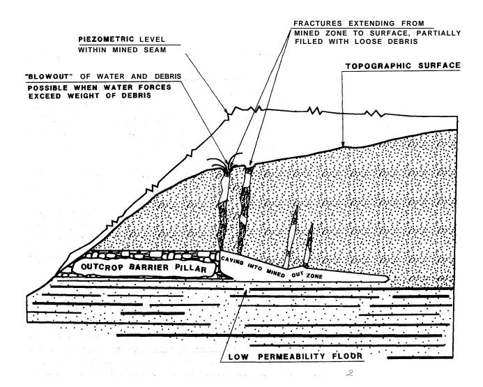
Figure 7.3 : Potential Hydraulic "Blowout" Location Source : U.S.D.I., Office of Surface Mining zone suggested the possibility of an entry into an abandoned underground mine. If excavation operations were to encounter a water-filled void, a rapid uncontrollable release of mine water would occur.
