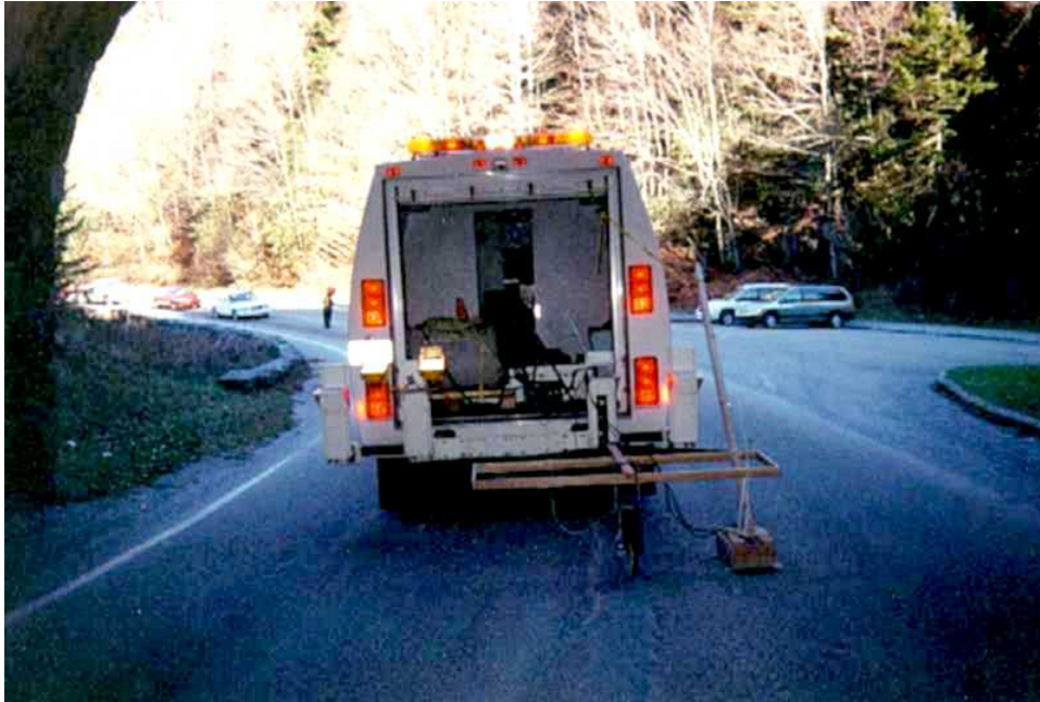
Figure 2. GPR survey in progress on the crown of the tunnel (top photograph) and the tunnel pavement (bottom photograph).
