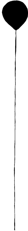
Figure 2. Sketch of experimental plume showing head and tail (chimney) parts. Drawn from photograph shown in Richards and others (1989, Fig. 2). The large bulbous plume head is fed by a much narrower tail or chimney. In this scale model, the plume head was 1.3 cm across. For the Yellowstone hot-spot track, we postulate that a plume head about 300 km across intercepted the lithosphere at 16 to 17 Ma and produced widespread volcanism and deformation, whereas from 10 Ma to present a much narrower chimney (tail) 10 to 20 km across has produced more localized volcanism, faulting, and uplift.
