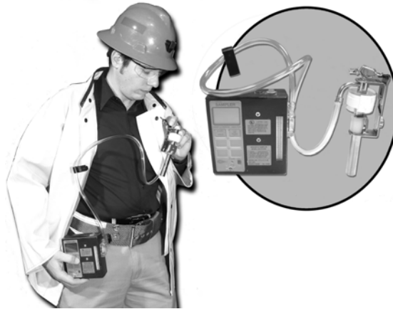
Figure 2-5 Respirable Dust Sampling Setup
