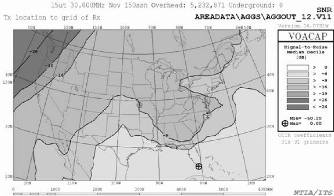
Figure 5-11: Aggregation example under high SSN conditions due to no underground devices and 5,232,871 overhead devices with maximum noise floor increase of 3 dB
