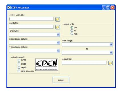
2. Type the folder path to the EDEN data files stored on your hard drive. This folder must contain one or more EDEN daily water level surface files (netCDF, .nc) and the EDEN DEM file for ground elevation (netCDF, .nc).
