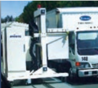
Portal VEDS Vehicular Explosive and Drug Sensor Can automatically scan all sizes of trucks and cars at fixed or temporary checkpoints for drugs or explosives.
