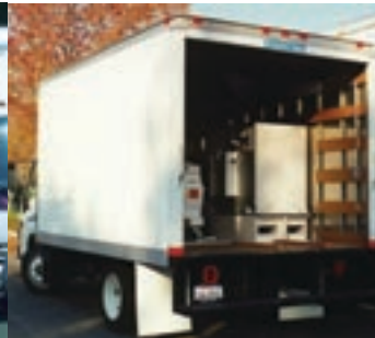
Mobile VEDS Vehicular Explosive and Drug Sensor Uniquely suited for automatic, material specific detection of significant amounts of explosives or drugs in vehicles.
