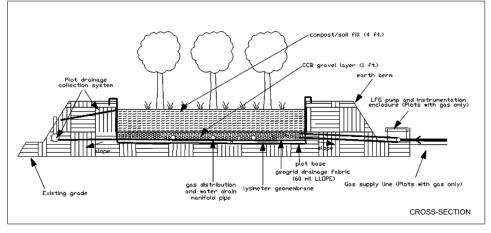
Each study plot consists of a gas distribution plenum (sandy-gravel) covered with a bioreactive layer of landfill cover soil mixed with compost. Lysimeters installed in each study plot are designed to capture infiltrating precipitation. Infiltrating precipitation is conveyed to water meters to measure volumes over time. A sub-base gravel mixture has been spread to form the base of each research plot. Landfill gas distribution piping is embedded into the base mixture.
