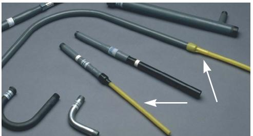
Most PE pipe manufacturers subscribe to the "Standard Dimension Ratio" (SDR) method of rating pressure piping. The SDR is the ratio of pipe diameter to wall thickness. An SDR 11 means the outside diameter (O.D.) of the pipe is eleven times the thickness of the wall.
