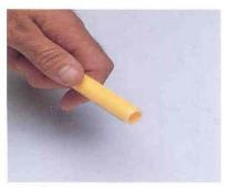
2Chamfer end of pipe using a chamfering tool.
