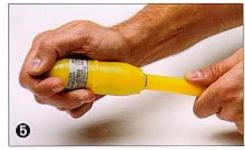
Stab the PE piping into the Permasert fitting so that the stab depth mark is visible:
