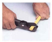
Check the pipe being used to be certain of correct pipe size. Cut pipe ends square.
