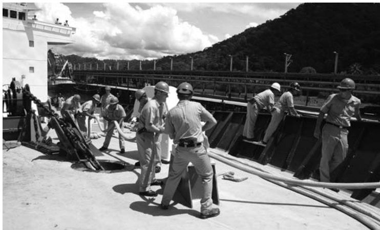
Berthing at the Costa Rica port of Golfito: Cadets man the lines and winches, supervised by California Maritime Academy faculty. This maneuver was completed without the use of tugs or shipboard thrusters.
