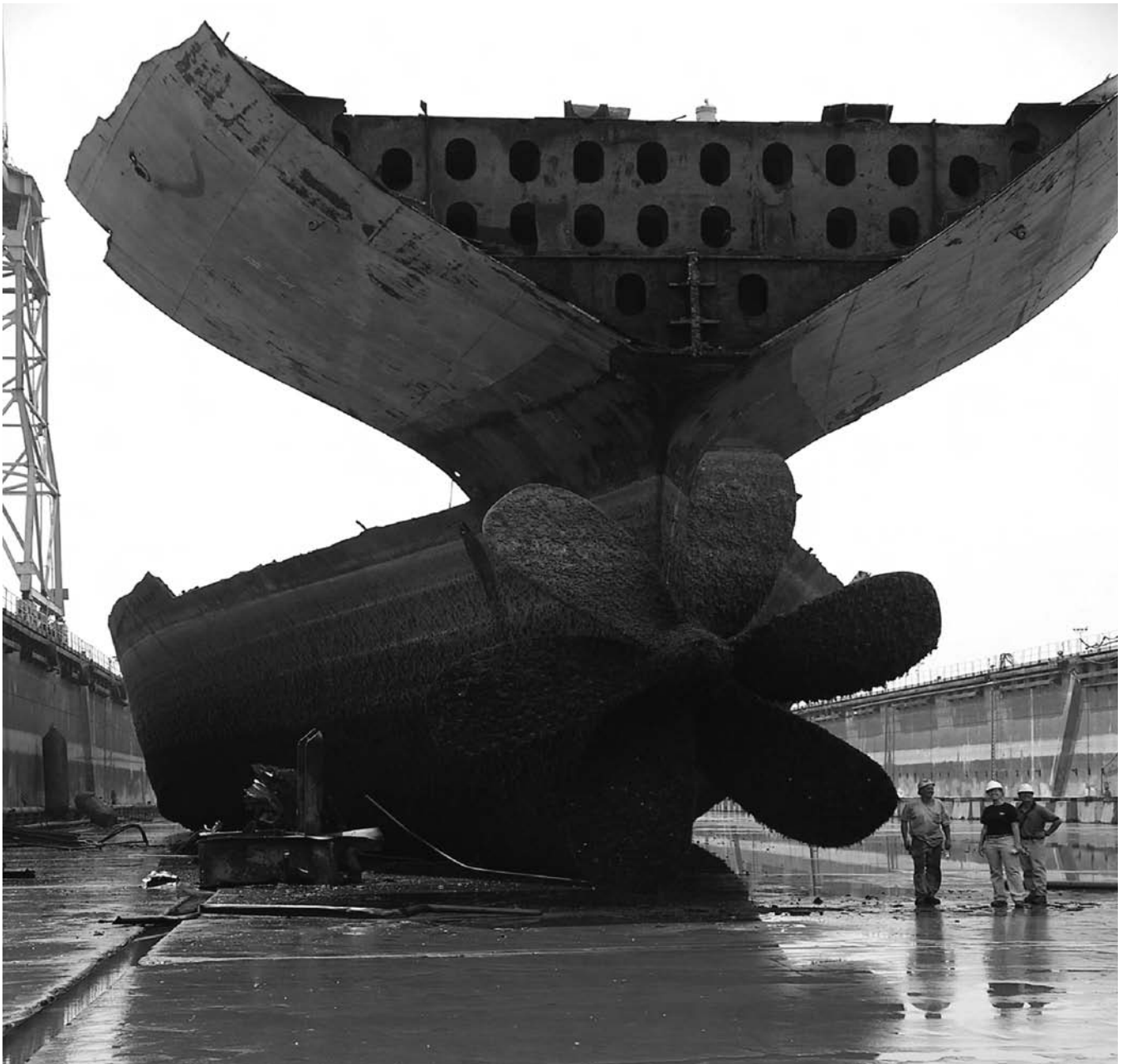
The remains of the Mormacmoon , which was dismantled at Sparrows Point, MD as part of the Ship Disposal Program. (Photo by David Condino)
