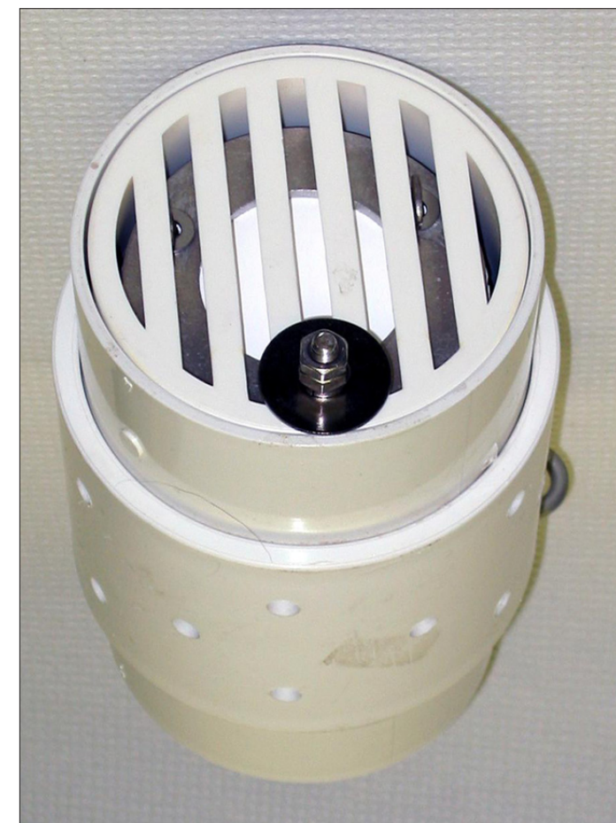
Plastic protective deployment canister containing six POCIS.
