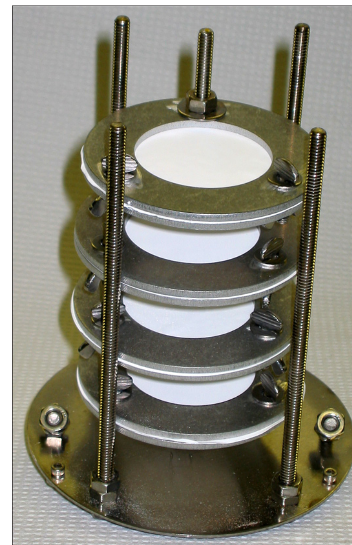
Four POCIS are shown mounted in a stainless steel deployment canister. Each POCIS has a sampling surface area of \approx 41\text{cm}^2 . Generally, POCIS of different configurations are deployed together inside a single protective canister to maximize the types of chemicals sampled. NOTE: The canister's outer protective screen was removed for picture clarity.
