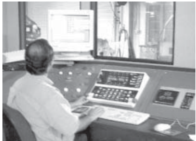
Figure 2: New Super Flow Dynamometer Control & Data Acquisition System
