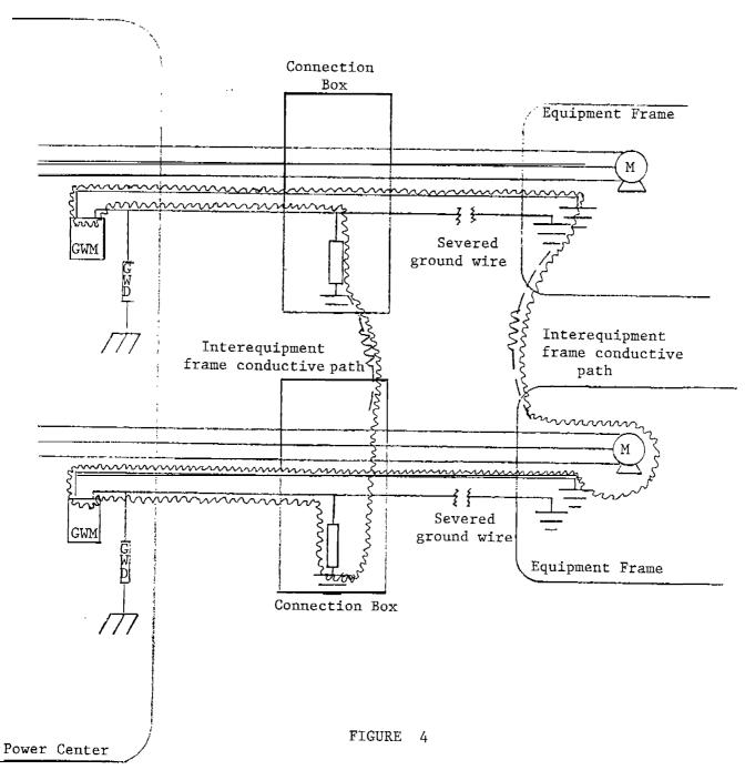
The ground wire monitor's control relays may remain energized when ground continuity is lost because some multiple sectionalized cable GWM/GWD configurations create complete monitoring loops which do not include the ground wires or parallel paths which make up the grounding circuits.
