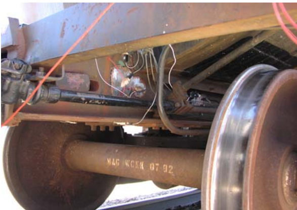
Figure 4. Placement of Strain Gages, Locations #21A-22A
