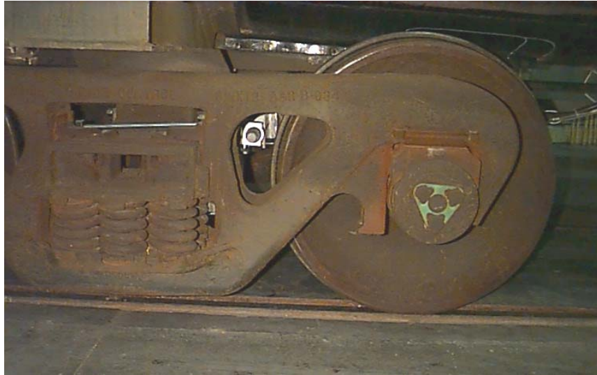
Figure 8. Bogie Group with Axle Generator Installed
