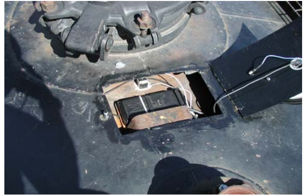
Figure 7. Independent Witness Data Acquisition Unit
