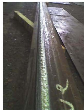
Photograph 10: Completed Rail Glaze
