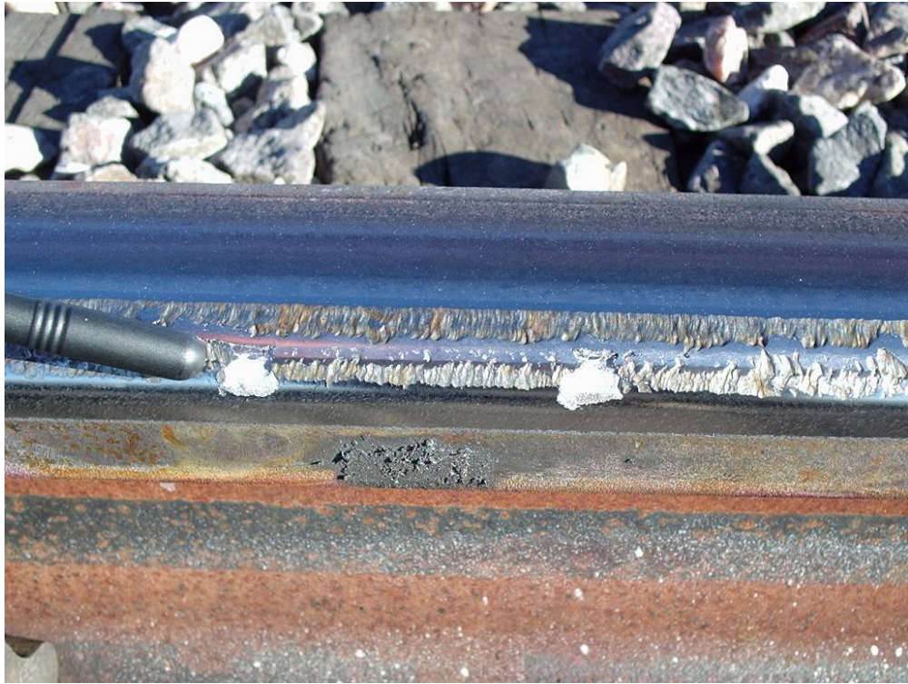
Figure 10. Closeup of the Same Location as Shown in Figure 9 After 1.2 MGT. Compare with Figure 17 on the Same Location After 5.6 MGT to Show Growth in Size of Spalling
