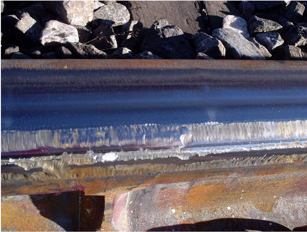
Figure 12. Closeup View of Thermite Weld (as Shown in Figure 11) in Laser-Treated Section After 1.2 MGT. Compare with Figure 20 at the Same Location After 5.6 MGT
