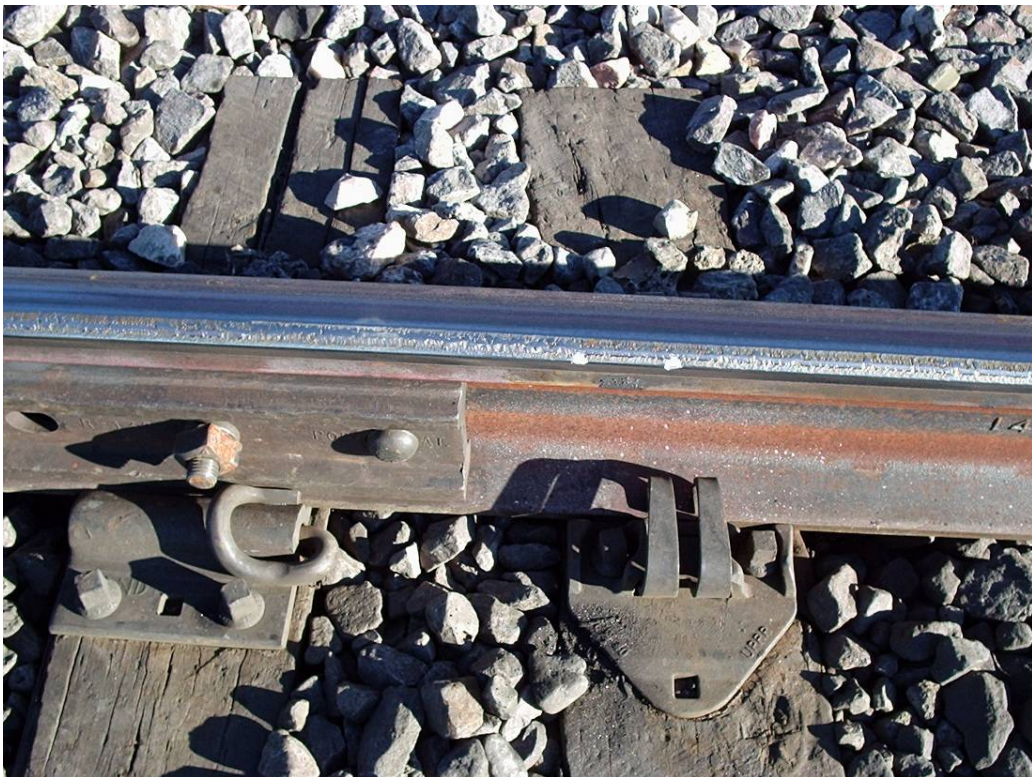
Figure 9. Two Chips on Gage Corner of Laser-Treated Rail After 1.2 MGT Compare with Figure 17 at the Same Location After 5.6 MGT
