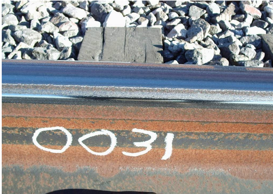
Figure 6. Control Rail After 1.2 MGT. Compare with Figures 14 and 15, Same Location After 5.6 MGT
