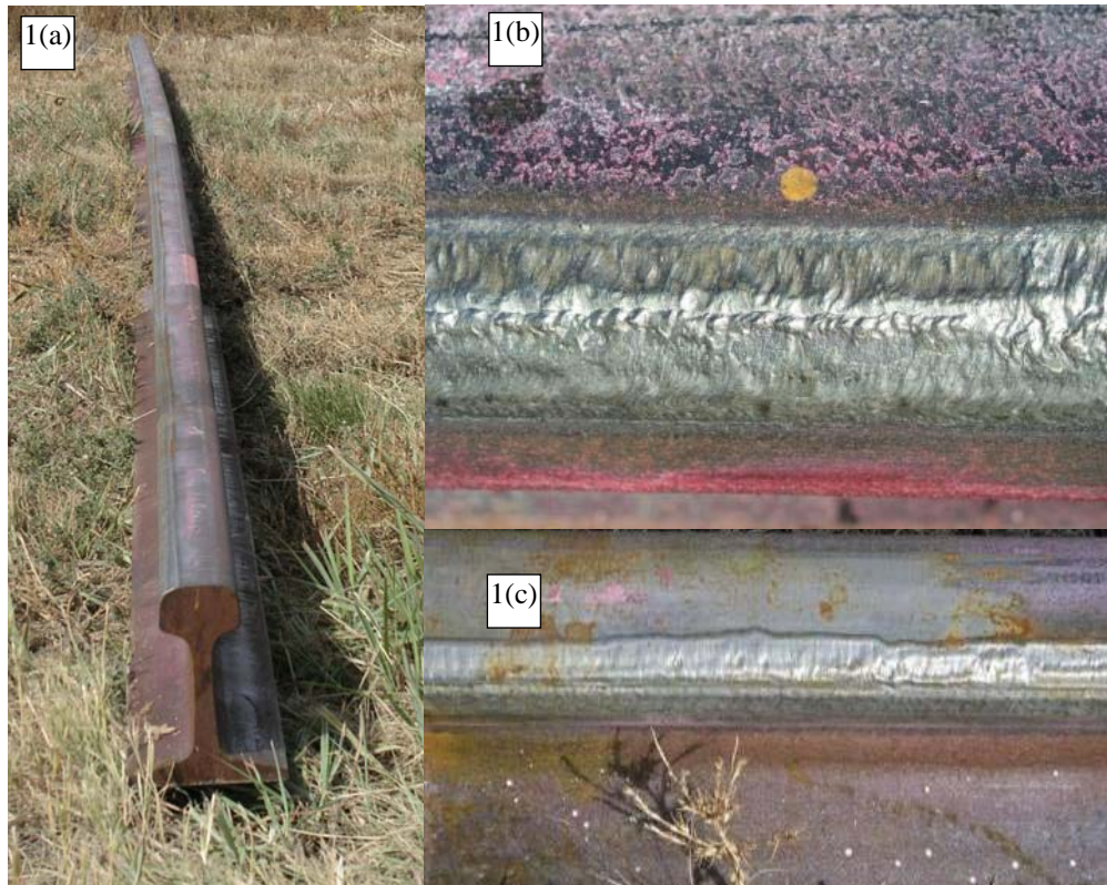
Figure A-1. Figure 1(a). Laser-Glazed Treated Rail, Figure A-1(b). Rough, and Figure A-1(c). Uneven Glazed-Treated Gages for the Untested Rail
