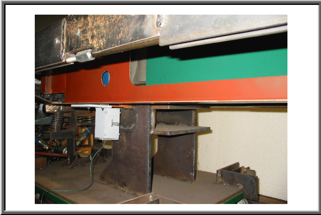
Figure 15. Electric coil system installed on the test bed
