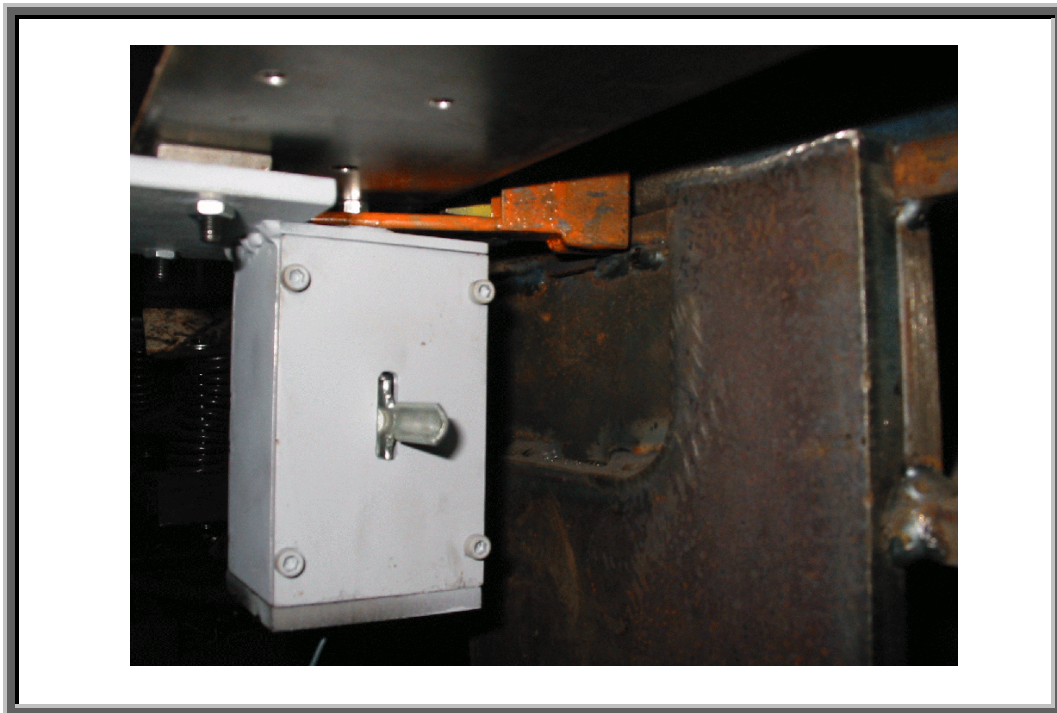
Figure 15. Electric coil system installed on the test bed
