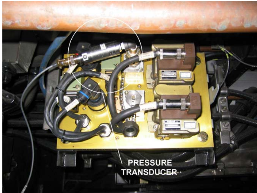
Figure 2.21. Pressure Transducer Used to Measure Brake Cylinder Pressure on Coach Car 3413
