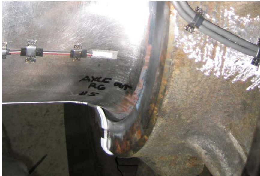
Figure 2.5. Strain Gage on Surface (Longitudinal Direction) of Axle with WABTEC/SAB-WABCO Supplied Discs
