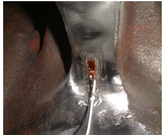
b) Gage Applied to Side of Spoke 3
