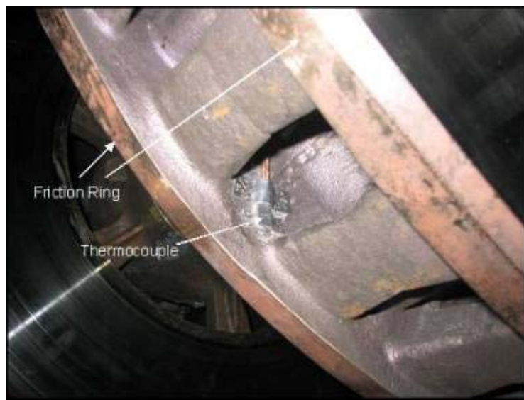
Figure 2.20. Thermocouple Applied on Back of Friction Ring of Instrumented WABTEC/SAB-WABCO Supplied Disc During Phase 1 of Acela Brake Disc Study
