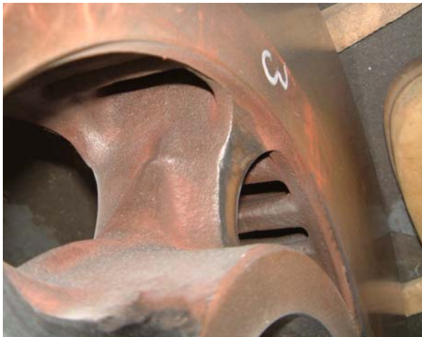
a) Spoke 3 Following Grinding on Side
