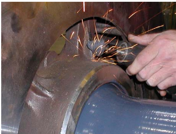
a) Spoke Grinding Process; Spoke to Left of Nut Unmodified
