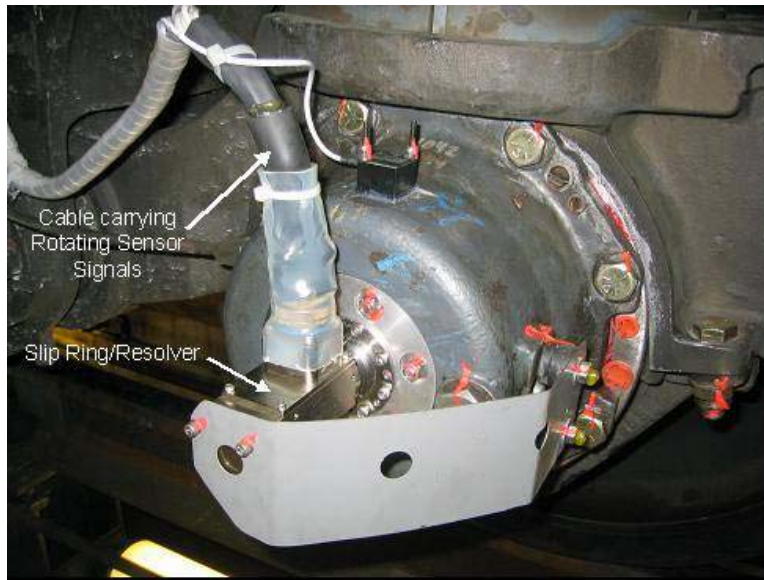
Figure 2.22. Slip Ring/Resolver Assembly with Wheel Position Output
