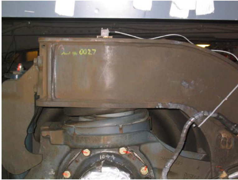
Figure 2.17. Tri-Axial Accelerometer on Truck Frame Over Primary Suspension of Knorr Test Axle During Phase 3 of Acela Brake Disc Study
