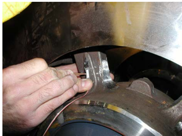
b) Gage Being Applied to Web on Spoke to Left of Nut
