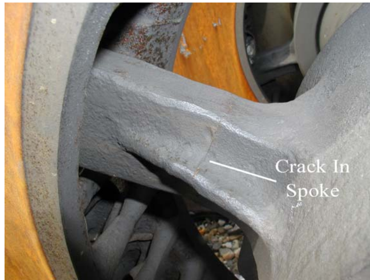
Figure 1.3. Example of a Crack in Spoke of WABTEC/SAB-WABCO Supplied Brake Disc Used on Acela Coach Car
