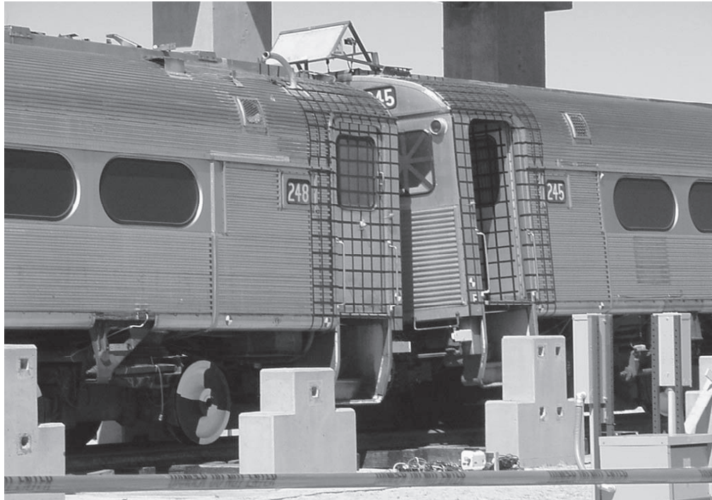
Figure 6. Sawtooth Lateral Buckling of Coupled Cars Observed in Two-Car Test
