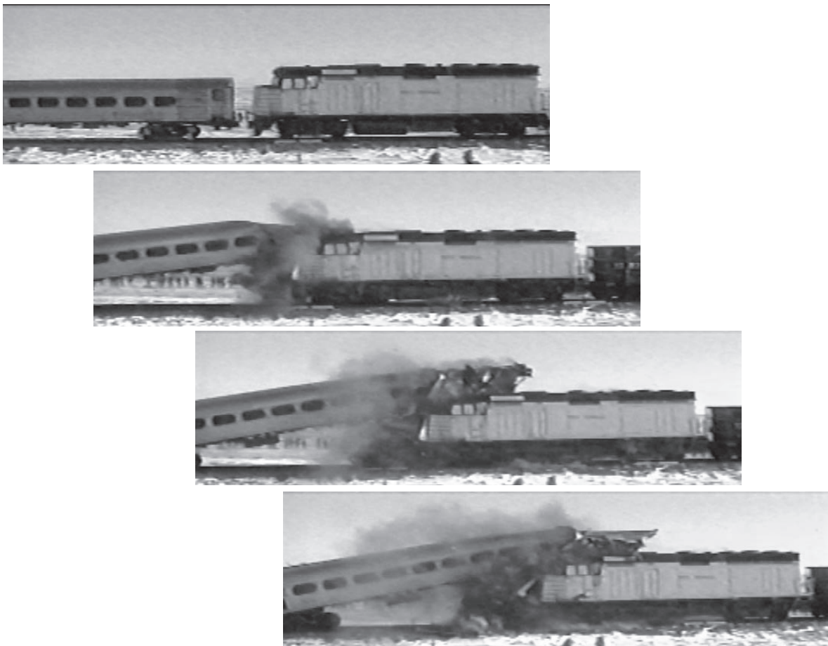
Figure 7. Override of Locomotive by Cab Car, Observed in Train-to-Train Test
