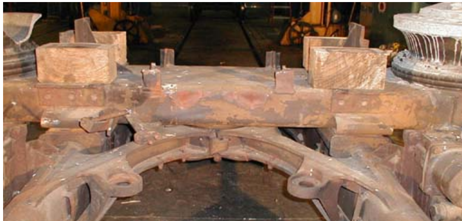
Figure B6-4. Forward Truck Detail Showing Indents from Bolster Beam Bracket Impact, Forward Looking Aft
