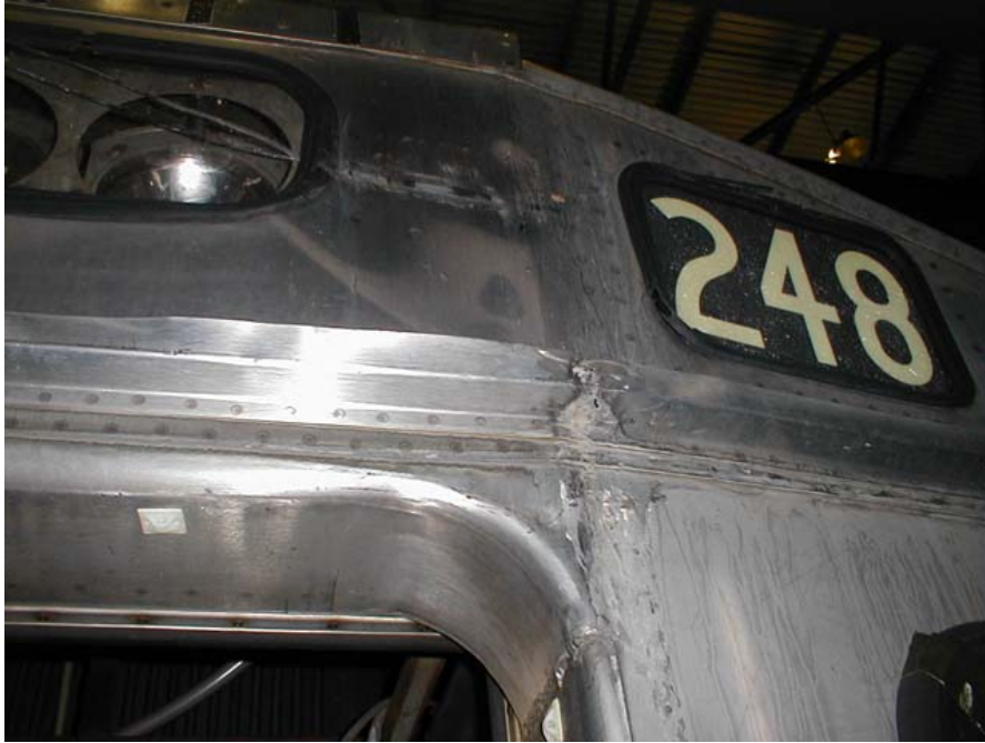
Figure B5-1. Damage above Rear Center Door - Impact of Rear Car Upper Step
