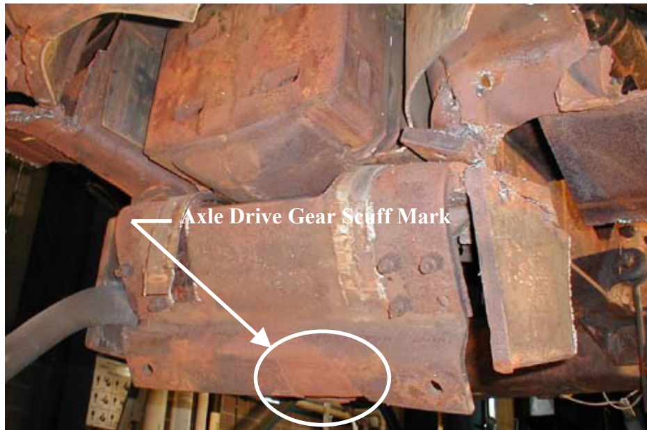
Figure 11. Pilot Attachment Hardware Detail—Axle Interaction
