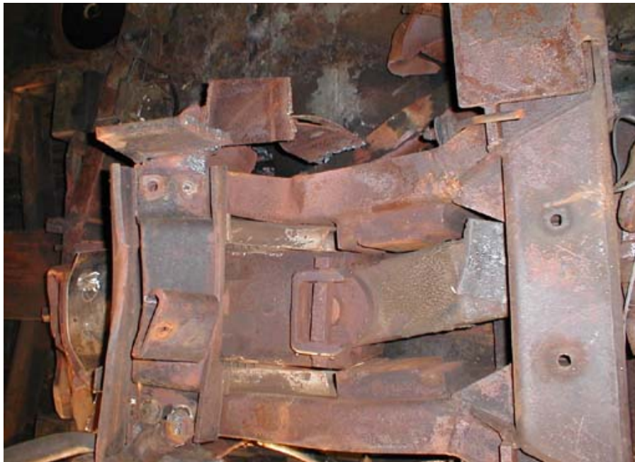
Figure B1-30. Forward Draft Sill, Coupler Shank, and Pilot Attachment From Below
