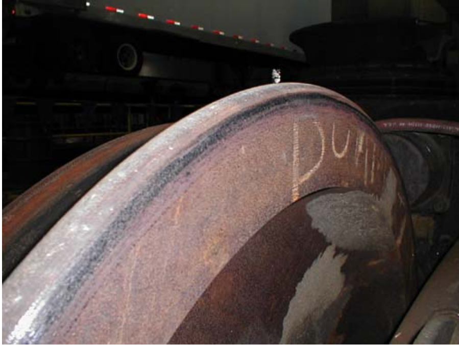
Figure B6-7. Wheel Burn - Polished Inside Surface on Right Front Wheel of the Forward Truck
