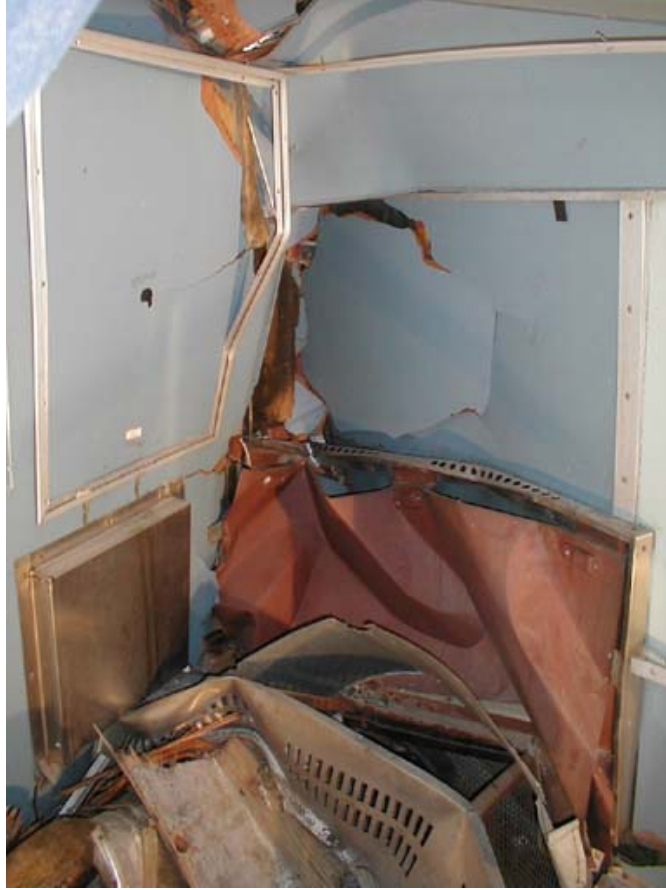
Figure B3-5. Inside Detail of Right Buckled Corner Aft of Bulkhead
