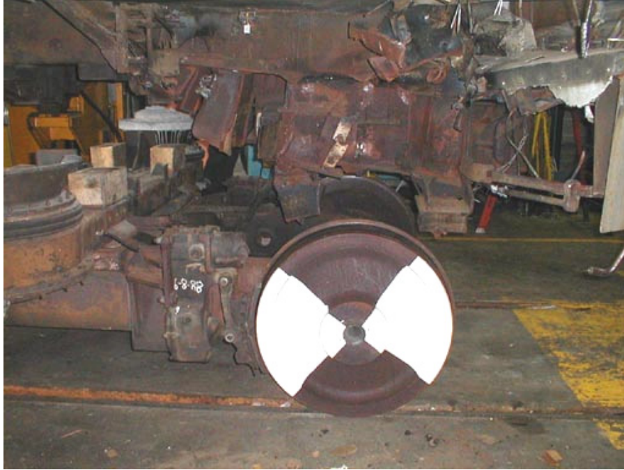
Figure B1-33. Draft Sill Position Relative to Truck—As Car was Being Lowered Back Onto Truck
