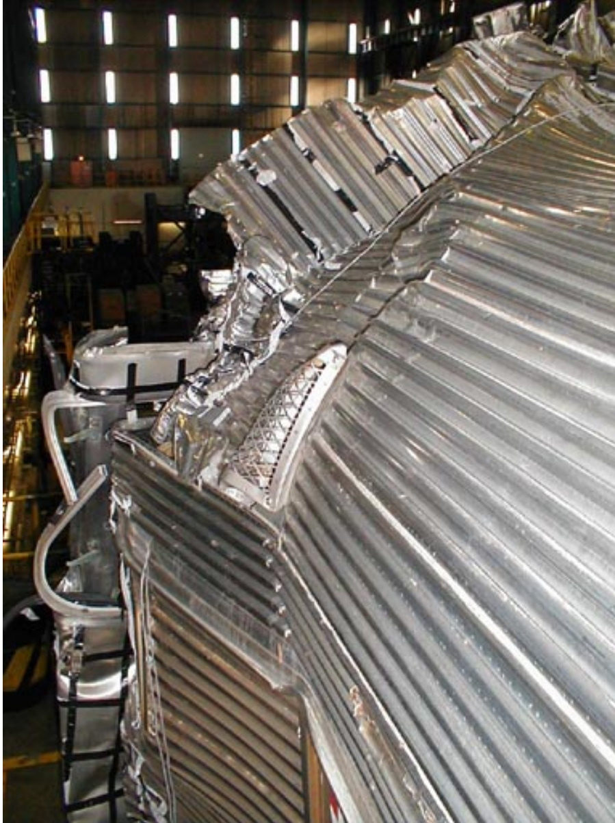
Figure B4-11. View of Upper Left-side Superstructure in Crush Zone, Looking Forward
