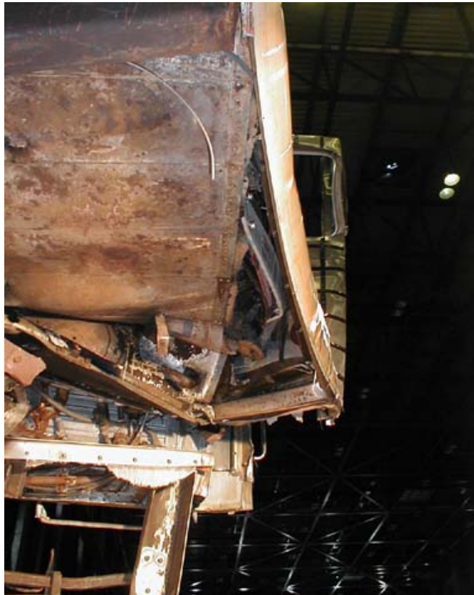
Figure B2-6. Forward Right-side Deformations - Buckling of the Side Sill and Floor Panels (Note Trap Door and Other Debris has been Removed)
