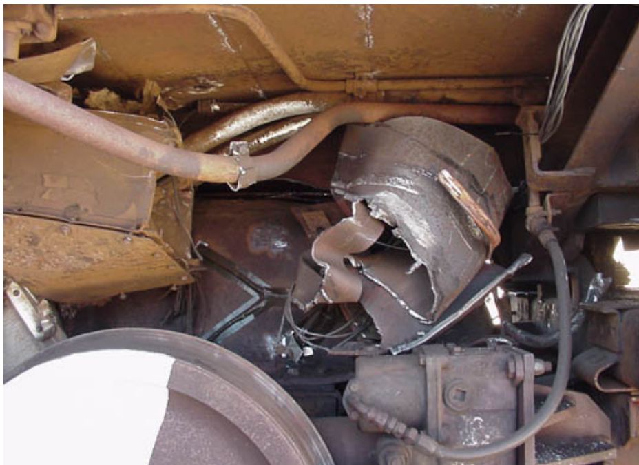
Figure 6. Left-side Draft Sill Collapse, Just After Test
