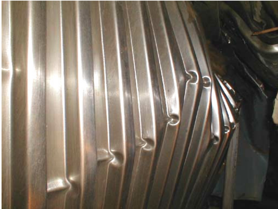
Figure B3-23. Same Buckle as Previous Picture from Slightly Different Point of View
