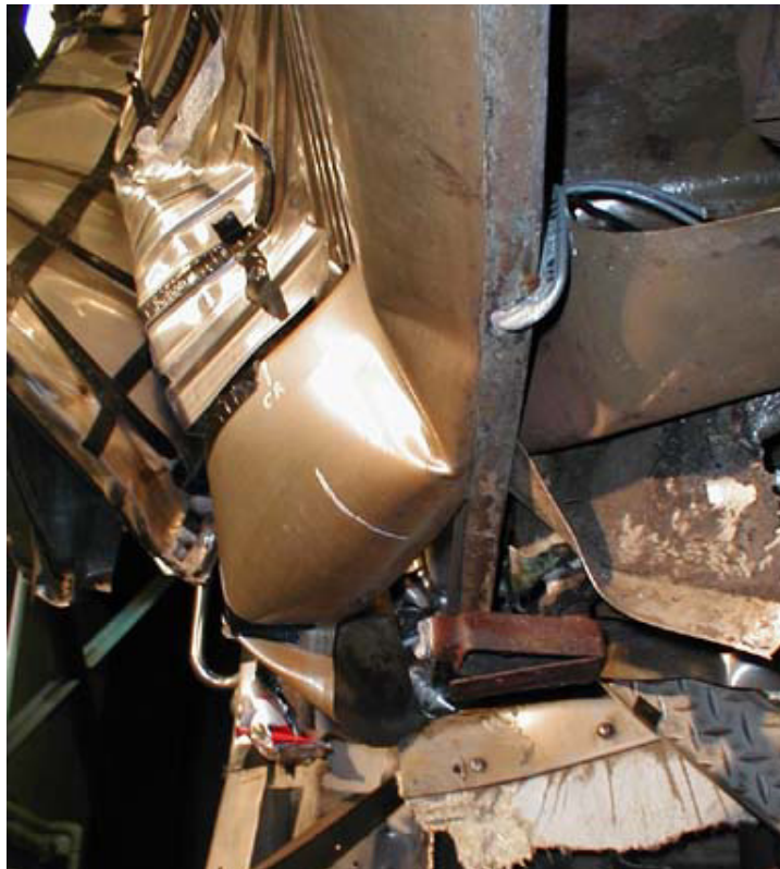
Figure B2-2. Left-side Sill Collapse Detail, from Below Looking Forward
