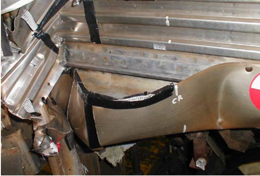
Figure B2-1. Detail of Deformed Side Sill Cover from Left Side Aft of Crushed Face (View of Side Sill is Obstructed by Cover)
