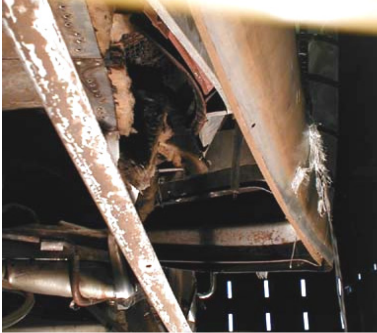
Figure B2-3. Right-side Sill Collapse Detail, from Below Looking Forward
