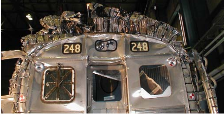
Figure B4-3. Front Top Face of Vestibule, Looking Up
