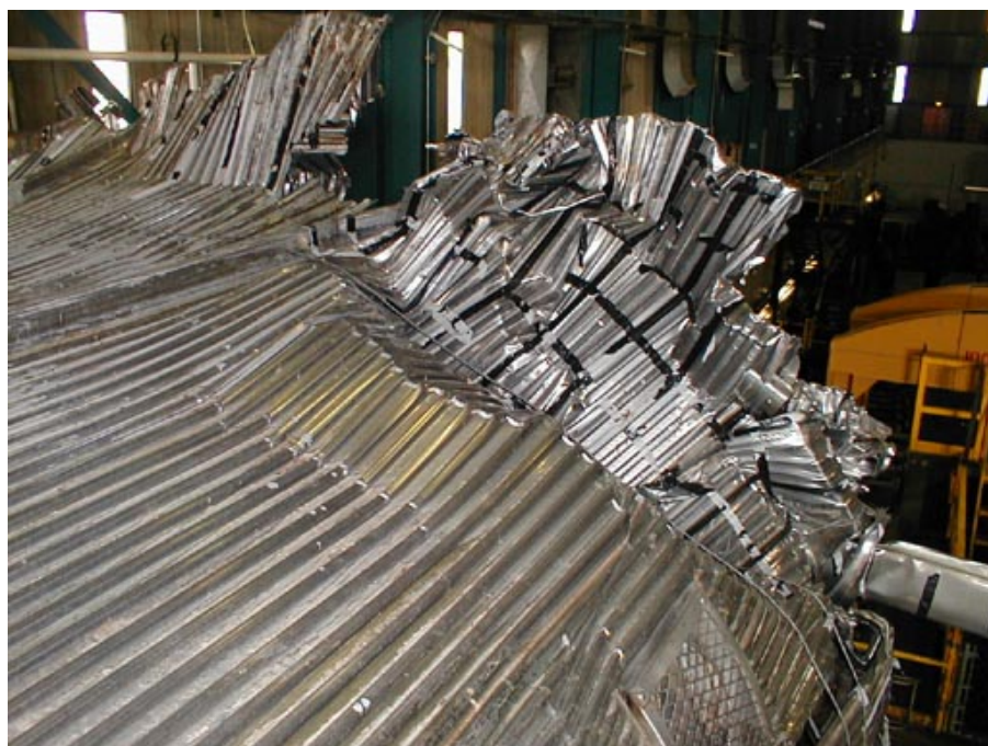
Figure B4-13. View of Upper Superstructure in Crush Zone, Looking Forward from Right
