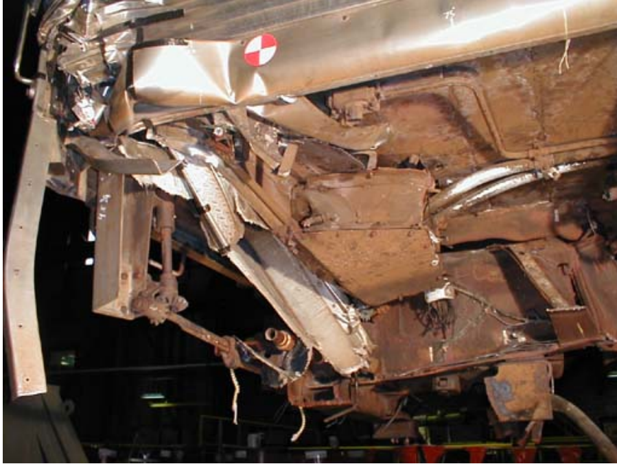
Figure B1-17. Front Draft Sill Collapse, Left Side
