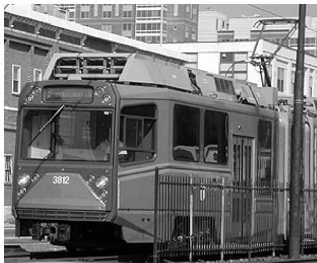
Figure 4 - MBTA Subway Car Showing the Front Ribbed Anticlimber
