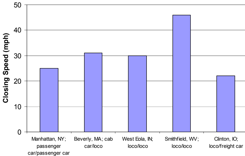
Figure 1 - Accident Examples in Which Override Occurred
