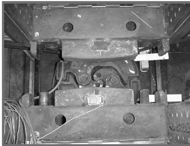
Figure 5 - Top View of U.S. Coupled Tight Lock Couplers (buffer elements have been removed.)
