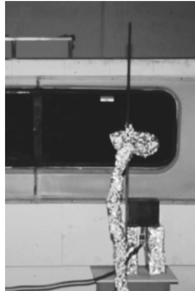
Figure A-16. Wall and Window Assembly Tests - General Configuration With Gas Sand Burner Ignition Source
