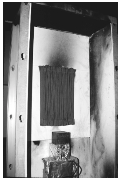
Figure A-13. Window Drape Assembly Tests (Extended and Contracted) - General Configuration with Gas Sand Burner Ignition Source
