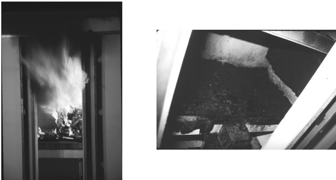
Figure A-25. Sleeping Compartment Economy Bedroom Lower Berth Test - During and After Trash Bag/Gas Sander Burner Ignition
