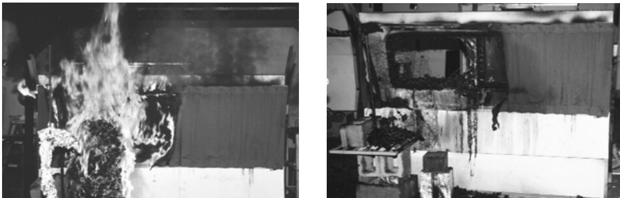
Figure A-34. Window and Drape Assembly Tests - During and After Trash Bag / Gas Sand Burner Ignition
