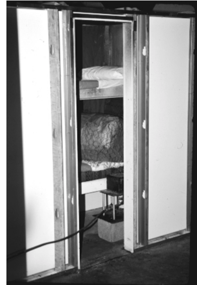
Figure A-10. Sleeping Compartment Economy Bedroom Assembly Tests - Upper and Lower Berths with Trash Bag/Gas Sand Burner Ignition Source
