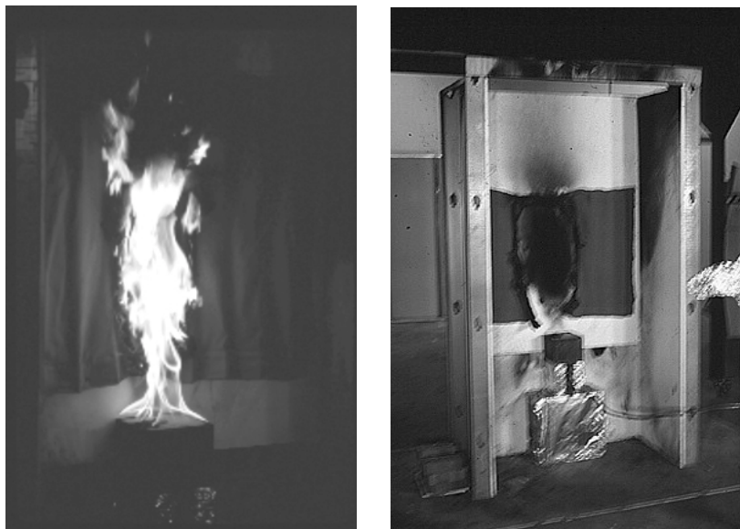
Figure A-29. Window Drape Assembly Test (Extended) - During and After Gas Sand Burner Ignition
