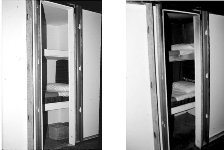
Figure A- 8 b. Sleeping Compartment Economy Bedroom Assembly Tests - General Configuration of Lower and Upper Berths
