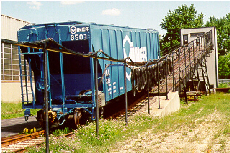
Figure 8. Hammer car on impact ramp
