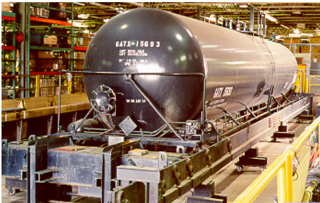
Figure 4. Tank car in the squeeze frame
