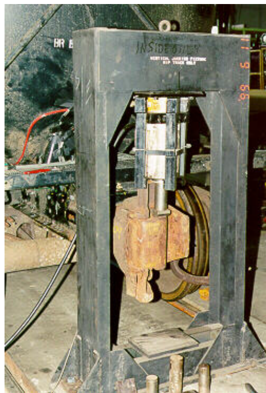
Figure 5. Coupler vertical load test
