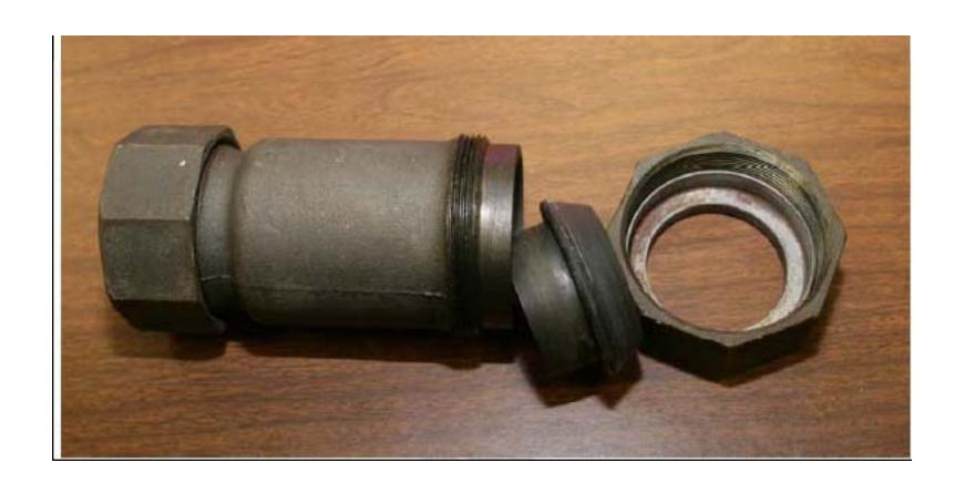
**Example of a Style 90 Type Dresser Coupling, Open Ended Barrel for View of Components**
