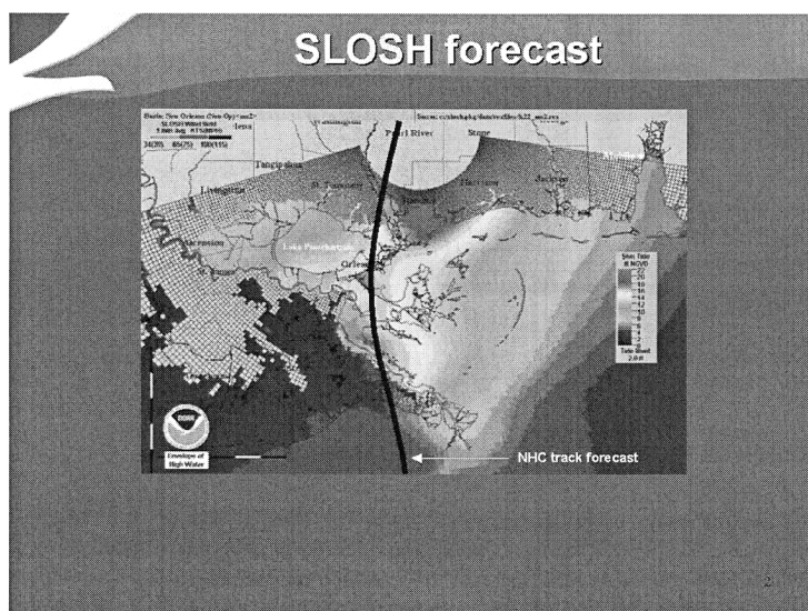
First SLOSH forecast based on the National Hurricane Center's forecast track of Hurricane Katrina. This information was available on the Internet at 9:20 a.m. CDT Sunday, August 29. The graphic depicts the predicted high water level above mean sea level. Additional SLOSH model forecasts were available following each advisory issued by the National Hurricane Center.
