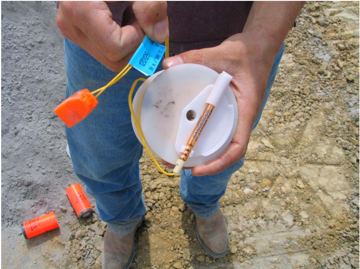
Figure 12 - Orca I-KON™ electronic detonator with unique ID tag
