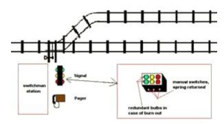
A partial solution to the hazard is to place signal lights in the line of sight of the operator that can communicate by color or code, the basic go, slow, stop signals. In this diagram the colors are used. The redundant light bulbs can greatly reduce erroneous communication in case of a burned-out bulb. The self centering, spring returned switches ensure that the operator knows that the switchman is in the proper location.
