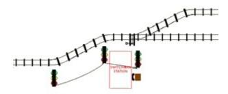
When the track entry is not straight, more than one of the signal lights, electrically linked, may need to be used to ensure that the operator has the signal in his line of
