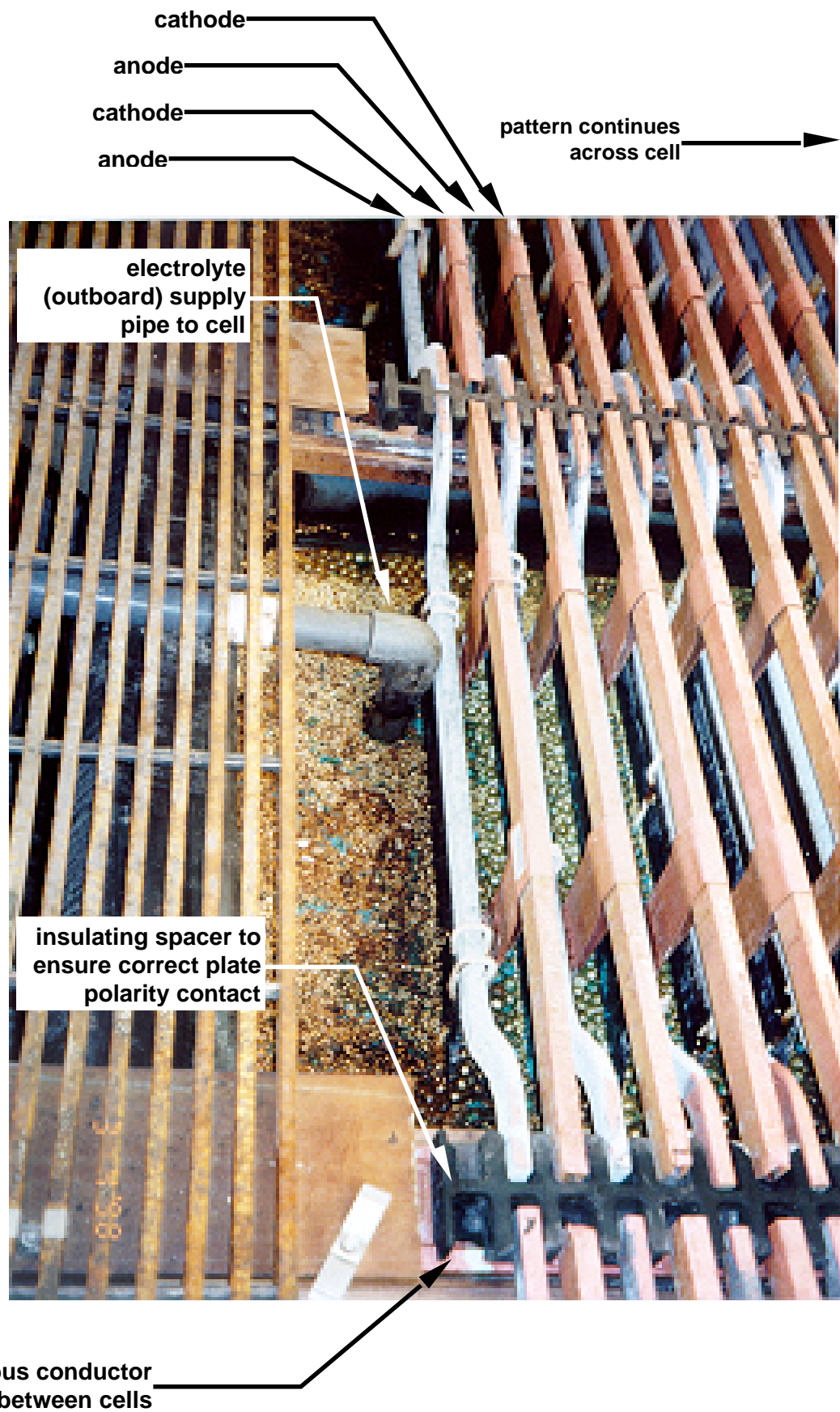
Figure-11 Basic features of operating cell
