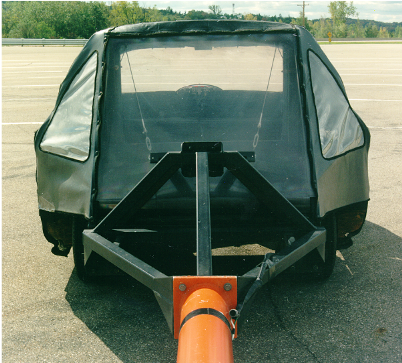
Figure 3-5 Close-up Front View of the Surrogate Target
