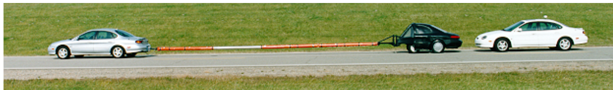
Figure 3-2 Side View of the Principal Other Vehicle (POV), Collapsible Beam, Surrogate Target and Subject Vehicle (SV)
