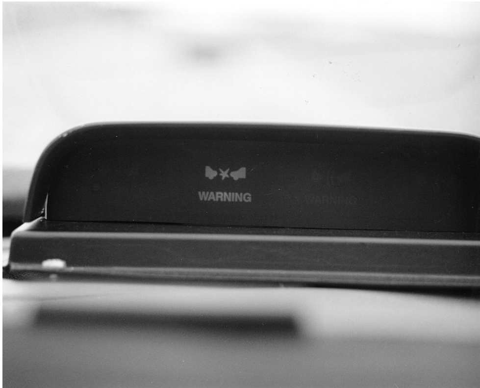
Figure 3-28 Illustrations of the High Head-Down Display (HHDD) and the Head-Up Display (HUD) Visual Crash Alerts
