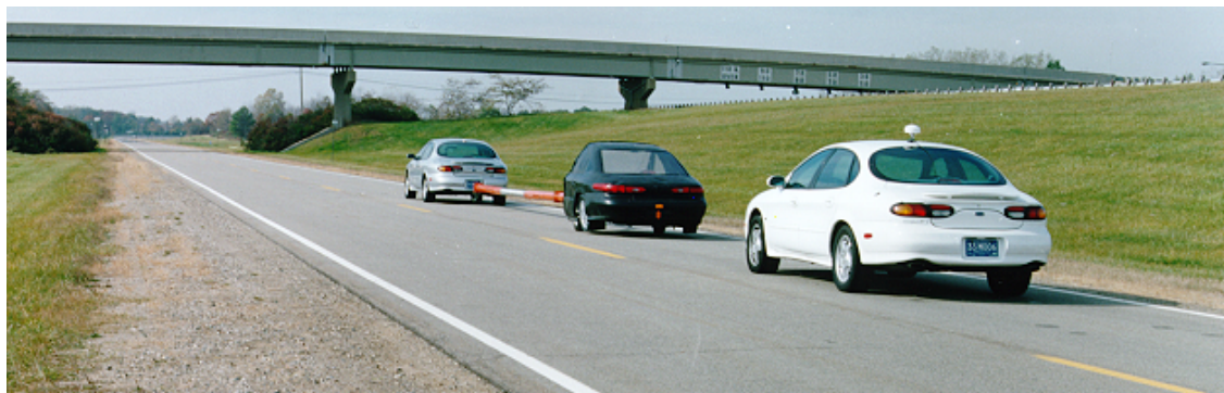
Figure 3-1 Side View of the Principal Other Vehicle (POV), Surrogate Target (Or Surrogate Lead Vehicle) and Subject Vehicle (SV), as well as an Illustration of the Test Track
