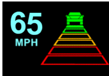
Figure 2.1. Relative size and position of the HUD images in the Delco driving simulator HUD. The alert-level indicator subtended a visual angle of approximately 1.5 x 2-deg of visual angle.
