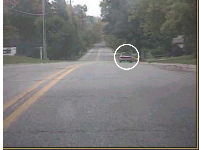
Figure 9.19 Straight Road False CIPS Event and Audible Alert Caused by Effect of Vertical Road Curvature on the Vision-Based Host Heading (Host Speed: 39 mph, CIPS Range: 50 meters)
