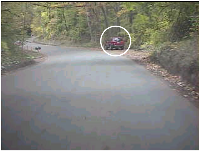
Figure 9.24 False CIPS Event and Audible Alert Due to an S-Curve (Host Speed: 32 mph, CIPS Range 54-33 meters)
