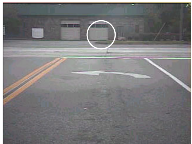
Figure 9.21 False CIPS Event Due to a T-Junction, No Audible Alert (Host Speed: 27 - 16 mph, CIPS Range: 67 to 53 meters)
