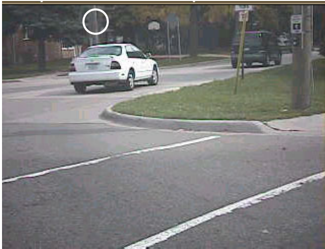
Figure 9.22 False CIPS Event Due to a Right Turn Followed by a Left Turn, No Audible Alert (Host Speed: 15 mph, CIPS Range: 28 to 30 meters)
