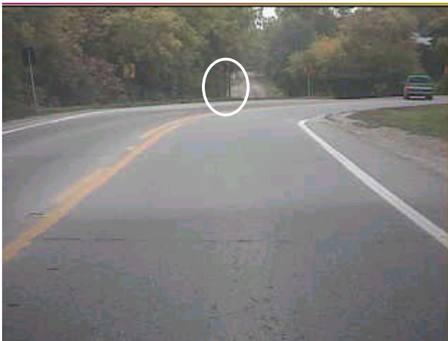
Figure 9.25 False CIPS Event and Audible Alert Due to a Curve Entry (Host Speed: 35-38 mph, CIPS Range 71- 54 meters)
