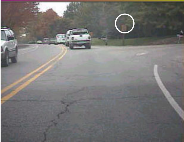
Figure 9.18 Straight Road False CIPS Event and Audible Alert Caused by Effect of Divergent Right Lane Marker on the Vision-Based Host Heading (Host Speed: 37 mph, CIPS Range: 42 meters)
