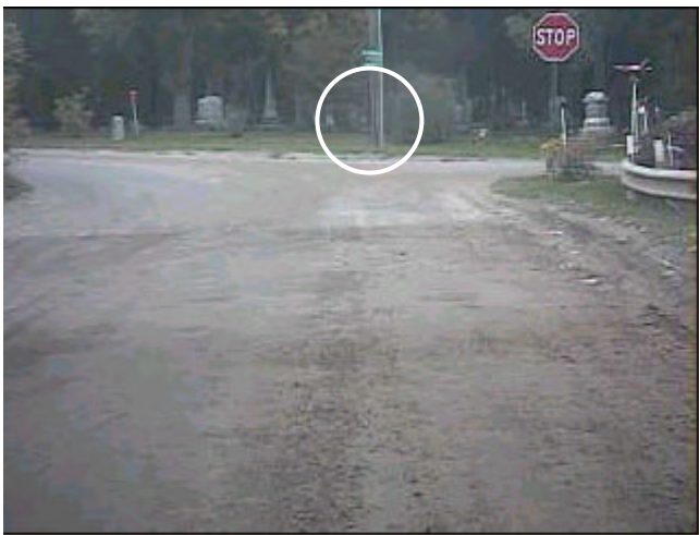
Figure 9.20 False CIPS Event Due to a Road Fork, No Audible Alert (Host Speed: 22 - 14 mph, CIPS Range: 76 to 24 meters)
