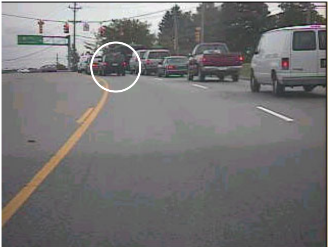
Figure 9.17 Valid CIPS Event on Intersection Approach (Host Speed: 45 – 10 mph, CIPS Range: 49 -15 meters)
