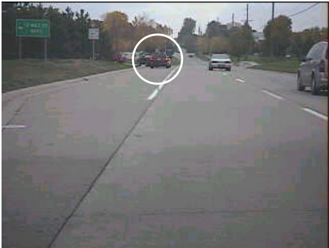
Figure 9.16 Valid CIPS Event on Host Lane Change Left into Adjacent Lane Stopped Vehicle (Host Speed: 35 – 15 mph, CIPS Range: 46 -12 meters)
