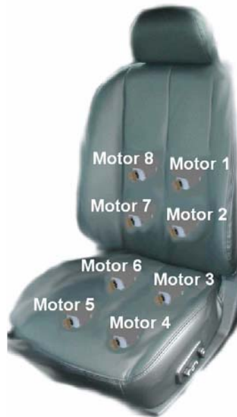
Figure 5.4.5 Haptic Seat – Transducer Distribution
