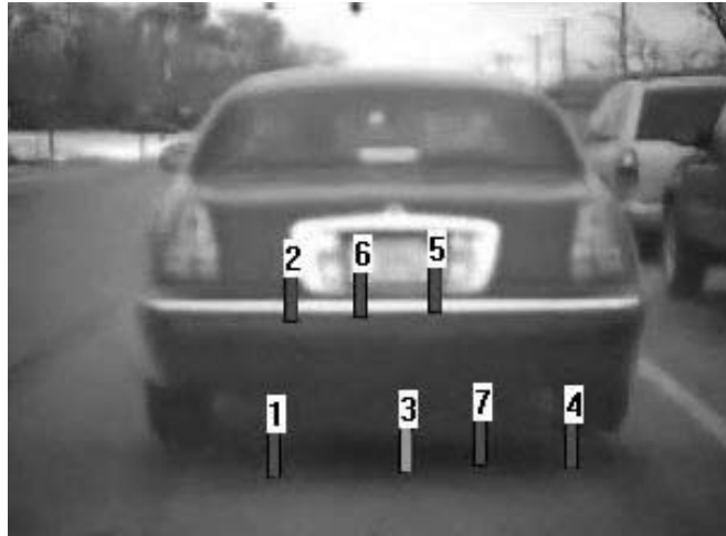
Figure 4-1 Example of Multiple Tracks Assigned to a Single Vehicle
