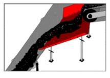
Chutes for section transfer belts need to be strong, but they can also be reusable and portable if they are made modular. It can save time and effort to have the pieces numbered for easy assembly and can also eliminate cutting and welding. The transfer chutes can be built with screw jacks so that two miners can handle the entire setup and assembly.
