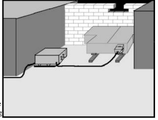
quick way to open the door remotely. The cable doesn't need to be any larger than an eighth of an inch. The pulleys and cable used to hang changeroom baskets will work very well for this application. Be sure to have a 'J' hook or other means to latch the door open after opening. Also, make sure that the cable and 'J' hook are located far enough outby to avoid smoke rollback. The mandoor should not be used as a regulator for the ventilation of the battery station.
