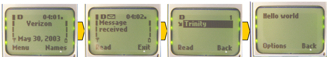
Figure A-1: The SMS Process on an Ericsson T68i in the USA T-Mobile Network
