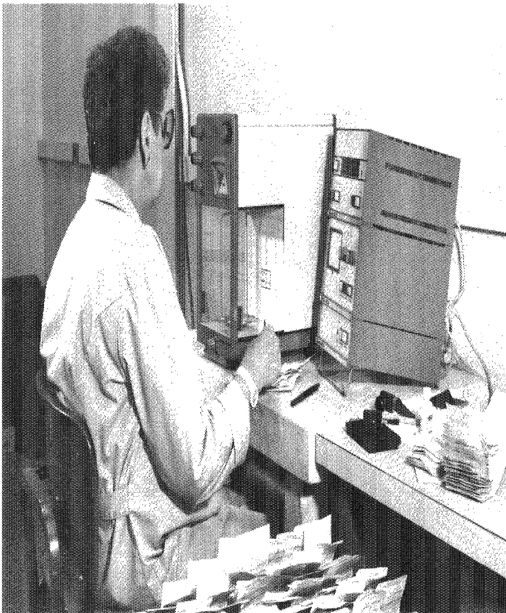
Figure 7. - Analytical balance used in manual weighing operation.
