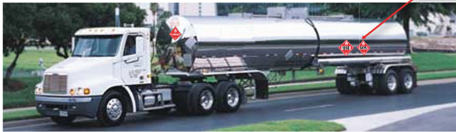
Sample Placarding/Marking Requirements* † Side view of single compartment multi-use cargo tank used for Gasoline, UN 1203 and Ethanol and Gasoline Mixtures, UN 3475
