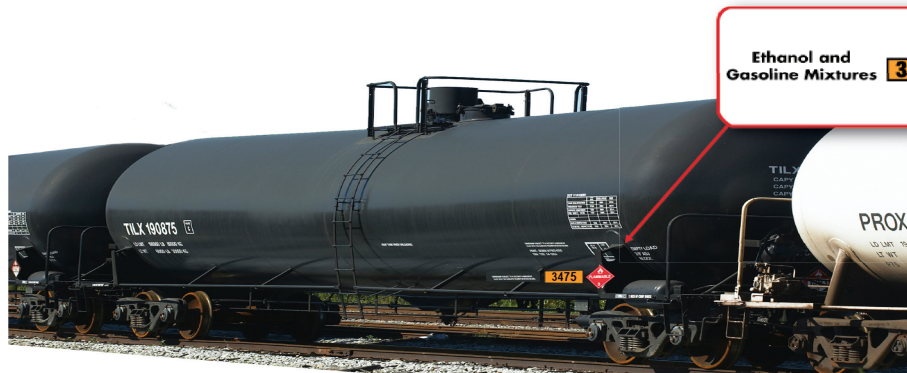
Sample Placarding/Marking Requirements* Side view of railcar used for Ethanol and Gasoline Mixtures, UN 3475
