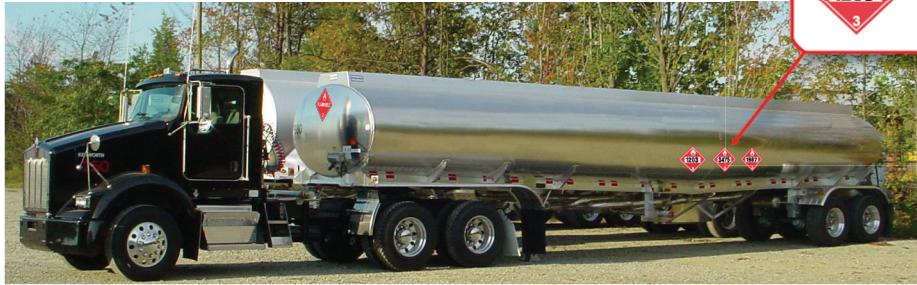
Sample Placarding/Marking Requirements* Side view of multi-compartment cargo tank carrying Gasoline, UN 1203; Ethanol and Gasoline Mixture, UN 3475; and Denatured Alcohol, NA 1987
