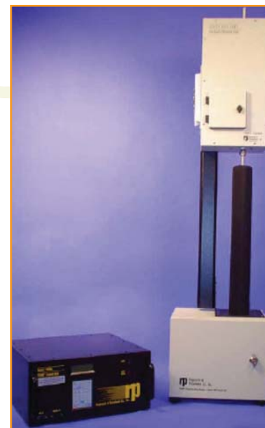
The Series 8500 FDMS™ unit has been selected by the California Air Resources Board as a California Approved Sampler for both \text{PM}_{2.5} and \text{PM}_{10} .
