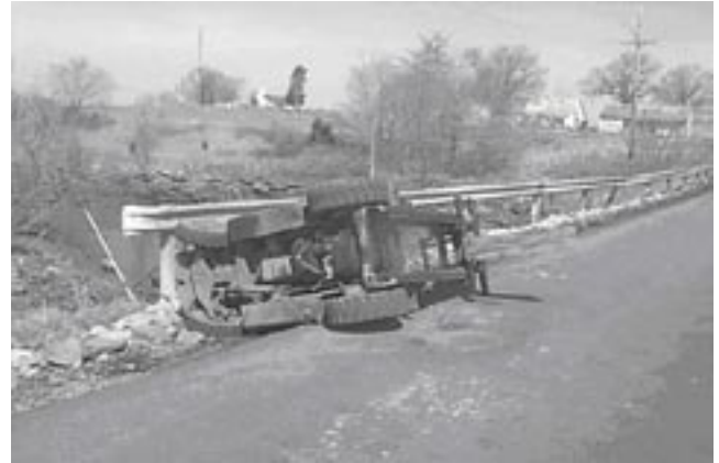
Figure 2. The forklift overturned when the left side tires traveled onto the shoulder
