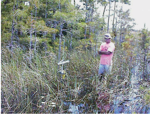
Figure 6. Typical Acoustic Doppler Velocity meter mounted on a specially designed wading rod.
