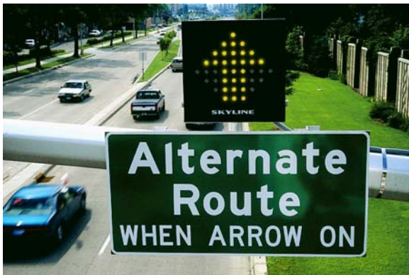
Figure 6-34 Dynamic Route Guidance Sign (Photo courtesy of the Minnesota DOT.)
