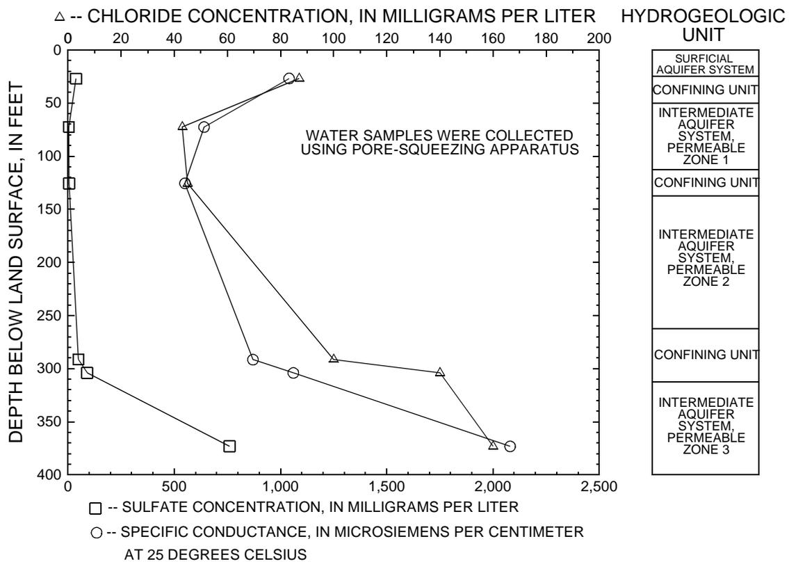
**Figure 50.** Chloride, sulfate, and specific-conductance values at selected depth intervals below land surface at the South Venice test well.
