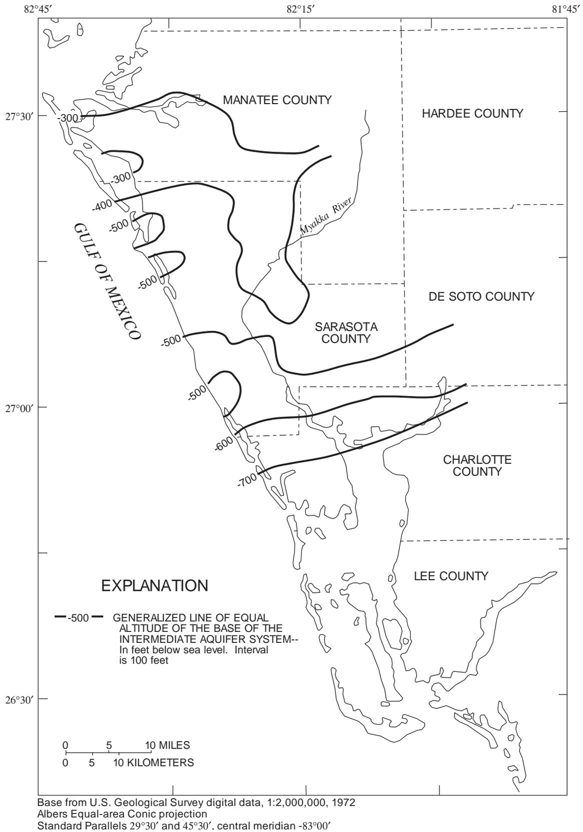
**Figure 18.** Generalized altitude of the base of the intermediate aquifer system in southwest Florida.
