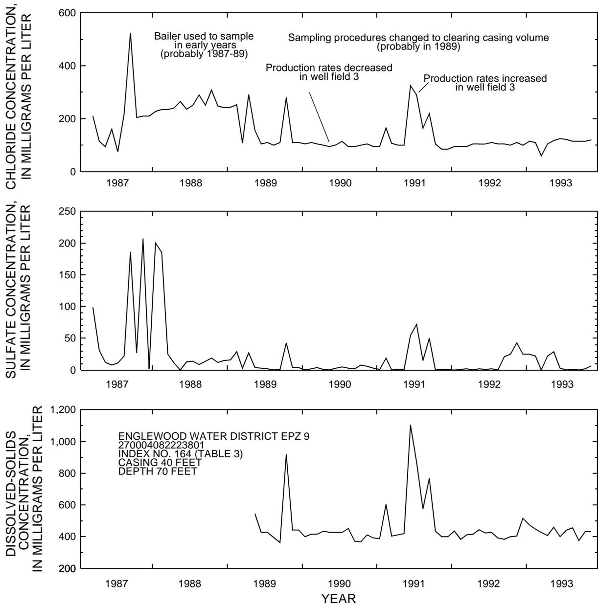
**Figure 41.** Chloride, sulfate, and dissolved-solids concentrations in water from intermediate aquifer system, permeable zone 1, at the Englewood Water District well EPZ 9, 1987-93. (Data collected by Englewood Water District personnel.)
