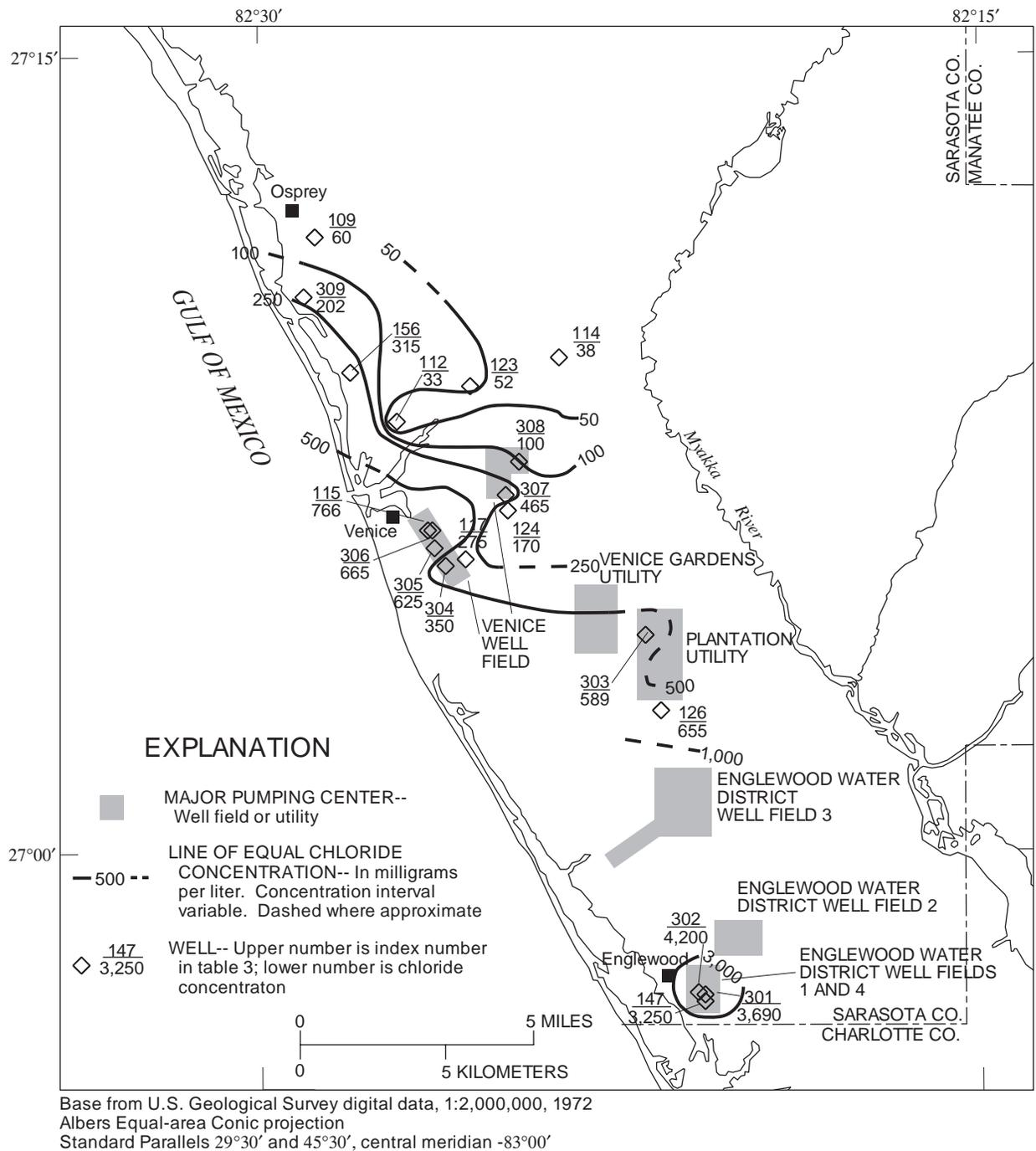
**Figure 37.** Chloride concentration in water from wells open to the intermediate aquifer system, permeable zone 3, in southwest Sarasota County.
