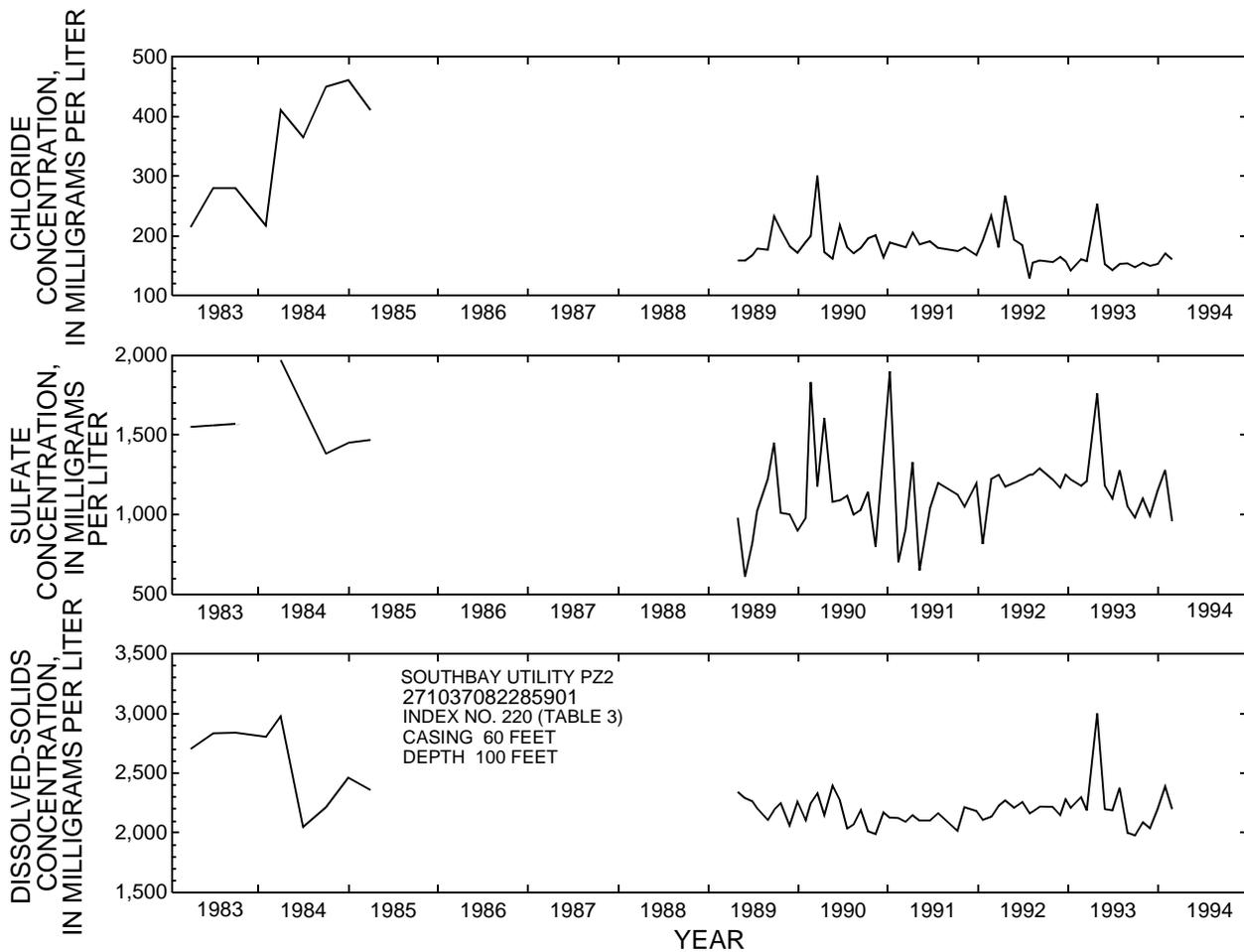
**Figure 44.** Chloride, sulfate, and dissolved-solids concentrations in water from intermediate aquifer system, permeable zone 2, at the Southbay Utility well PZ2, 1983-94. (Data collected by Southbay Utility personnel.)
