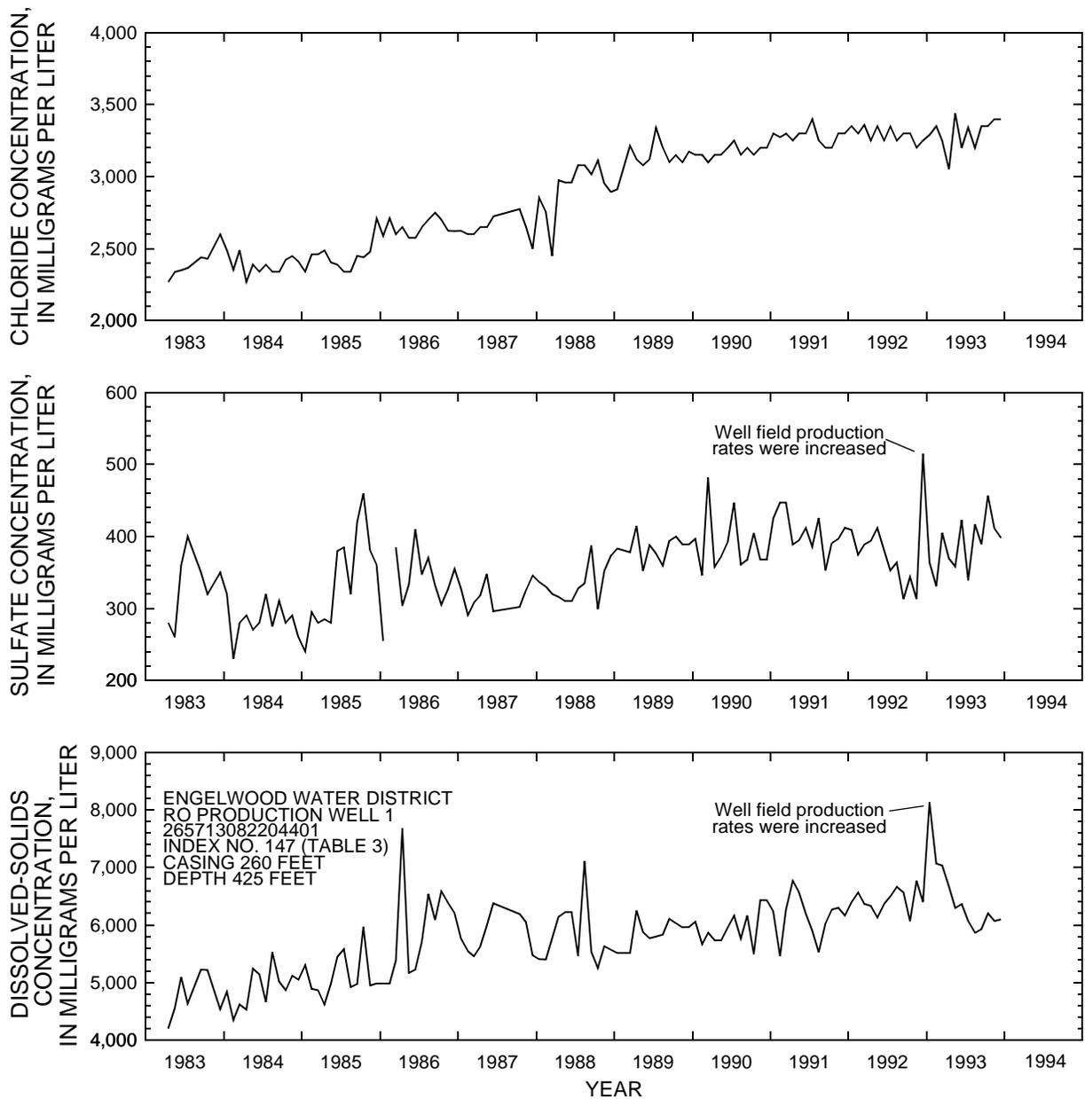
**Figure 45.** Chloride, sulfate, and dissolved-solids concentrations in water from intermediate aquifer system, permeable zone 3, at the EWD RO Production well 1, 1983-93. (Data collected by Englewood Water District personnel.)
