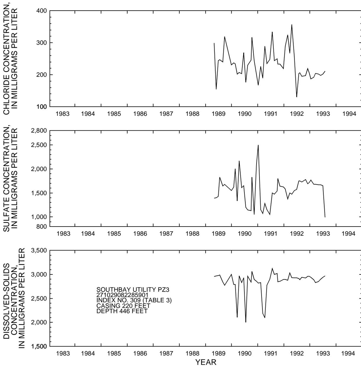
**Figure 48.** Chloride, sulfate, and dissolved-solids concentrations in water from intermediate aquifer system, permeable zone 3, at the Southbay Utility well PZ3, 1989-93. (Data collected by Southbay Utility personnel.)
