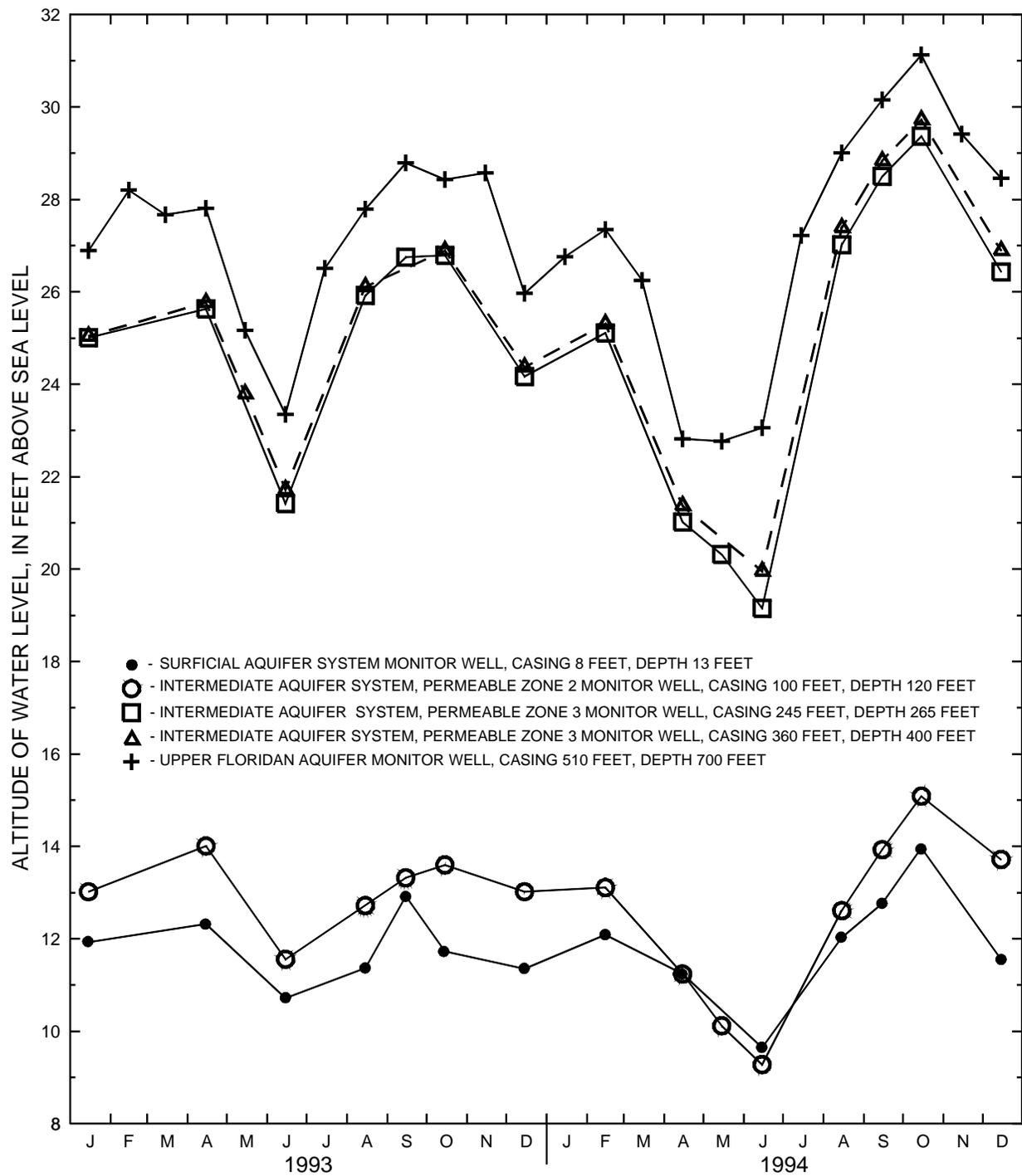
**Figure 54.** Water levels in the surficial, intermediate, and Upper Floridan aquifer monitor wells at ROMP TR 5-2, January 1993 to December 1994.
