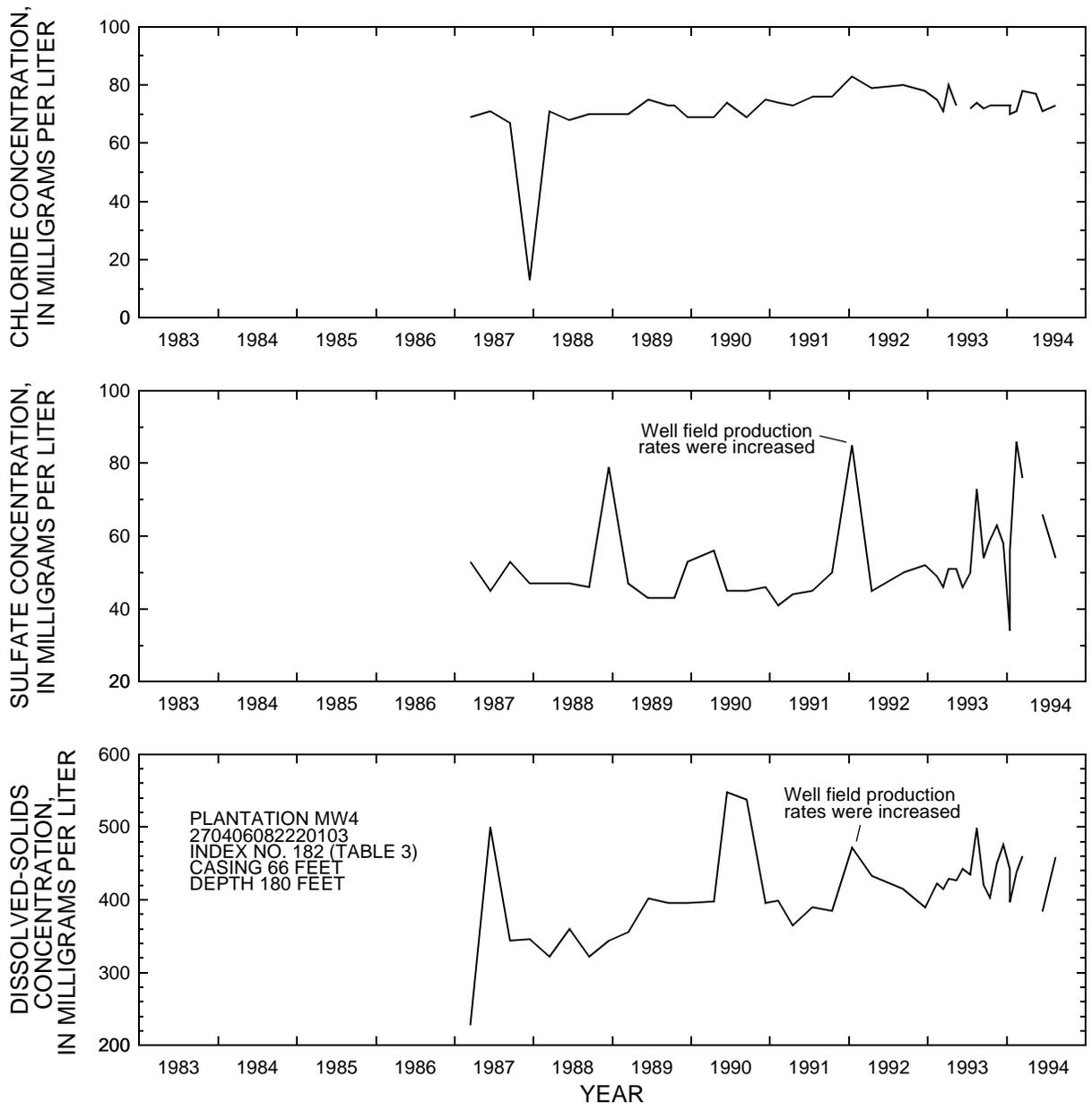
**Figure 43.** Chloride, sulfate, and dissolved-solids concentrations in water from intermediate aquifer system, permeable zone 2, at the Plantation monitor well MW4, 1987-94. (Data collected by Plantation personnel.)
