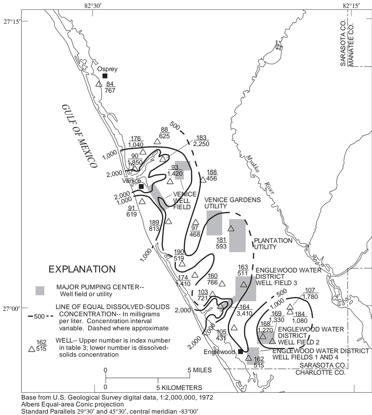
**Figure 31.** Dissolved-solids concentration in water from wells open to the intermediate aquifer system, permeable zone 1, in southwest Sarasota County.
