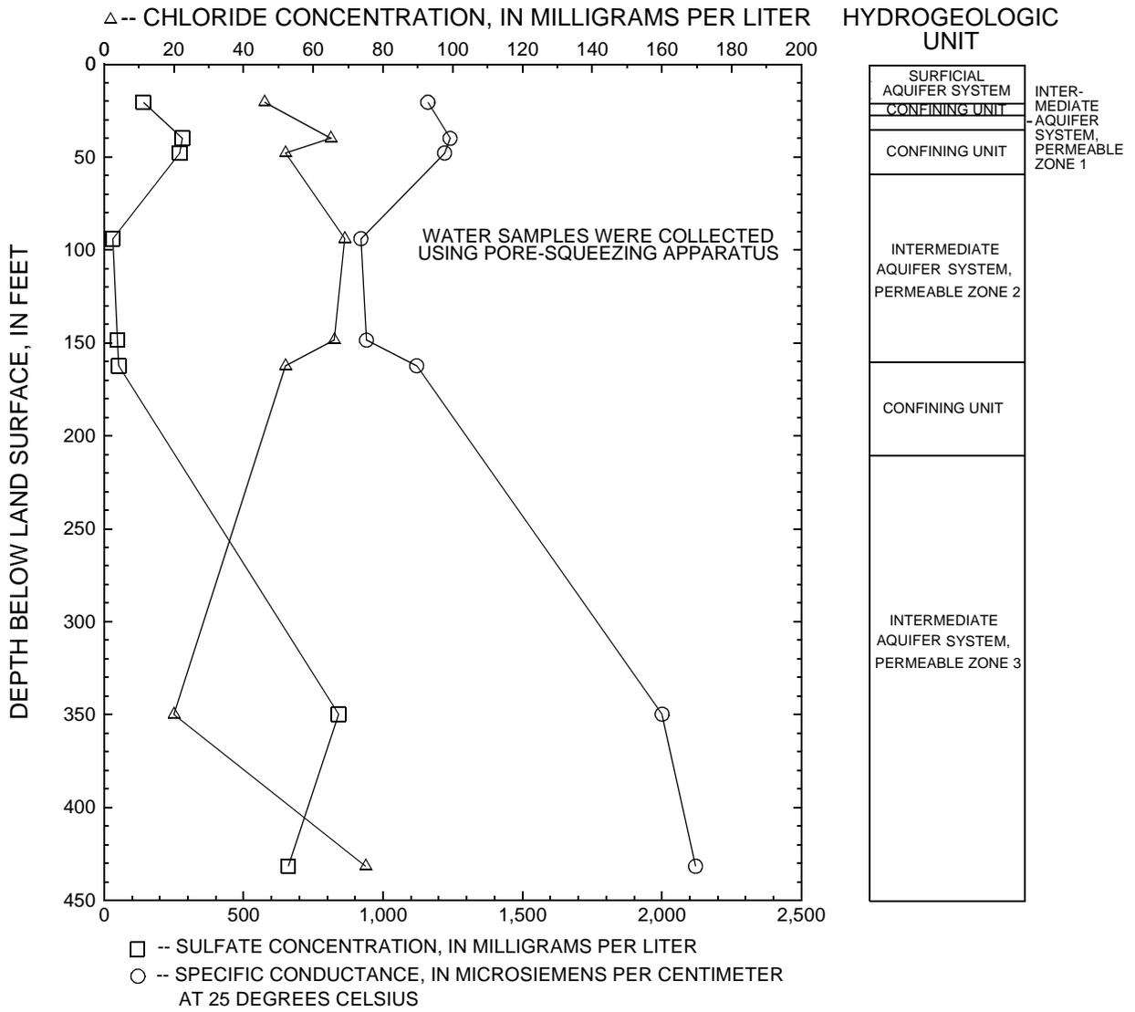
**Figure 49.** Chloride, sulfate, and specific-conductance values at selected depth intervals below land surface at the Carlton Reserve test well.
