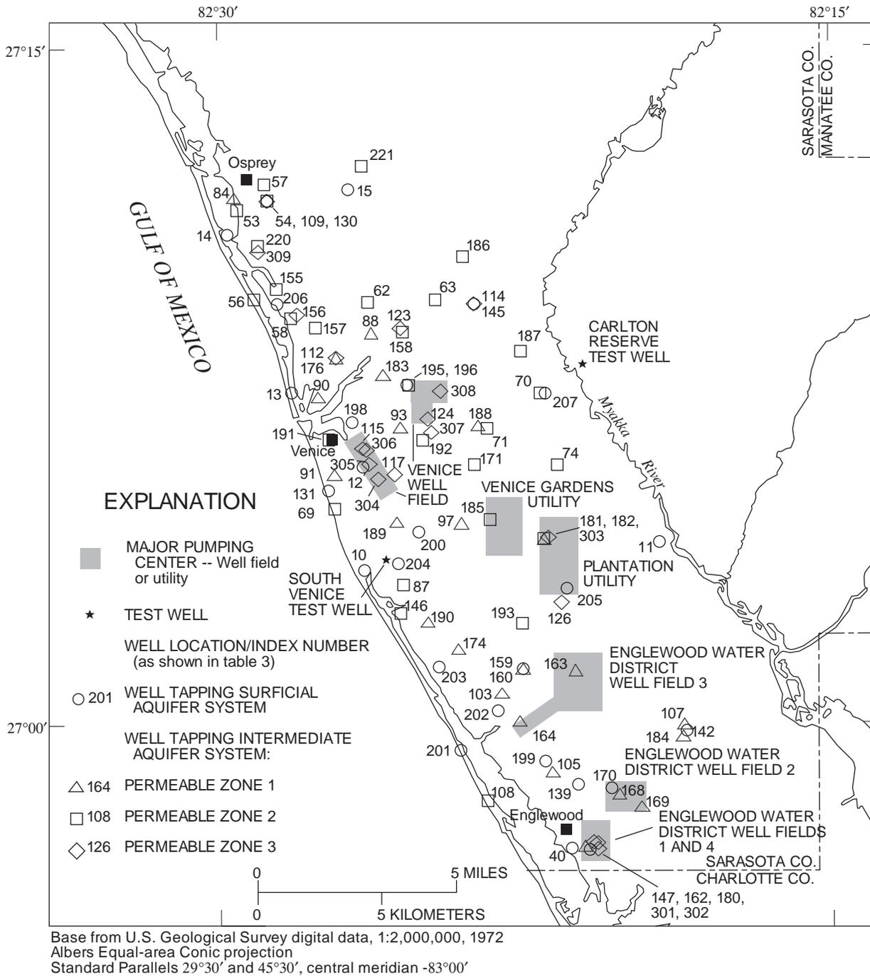
**Figure 24.** Surficial and intermediate aquifer system ground-water quality monitor wells in southwest Sarasota County.
