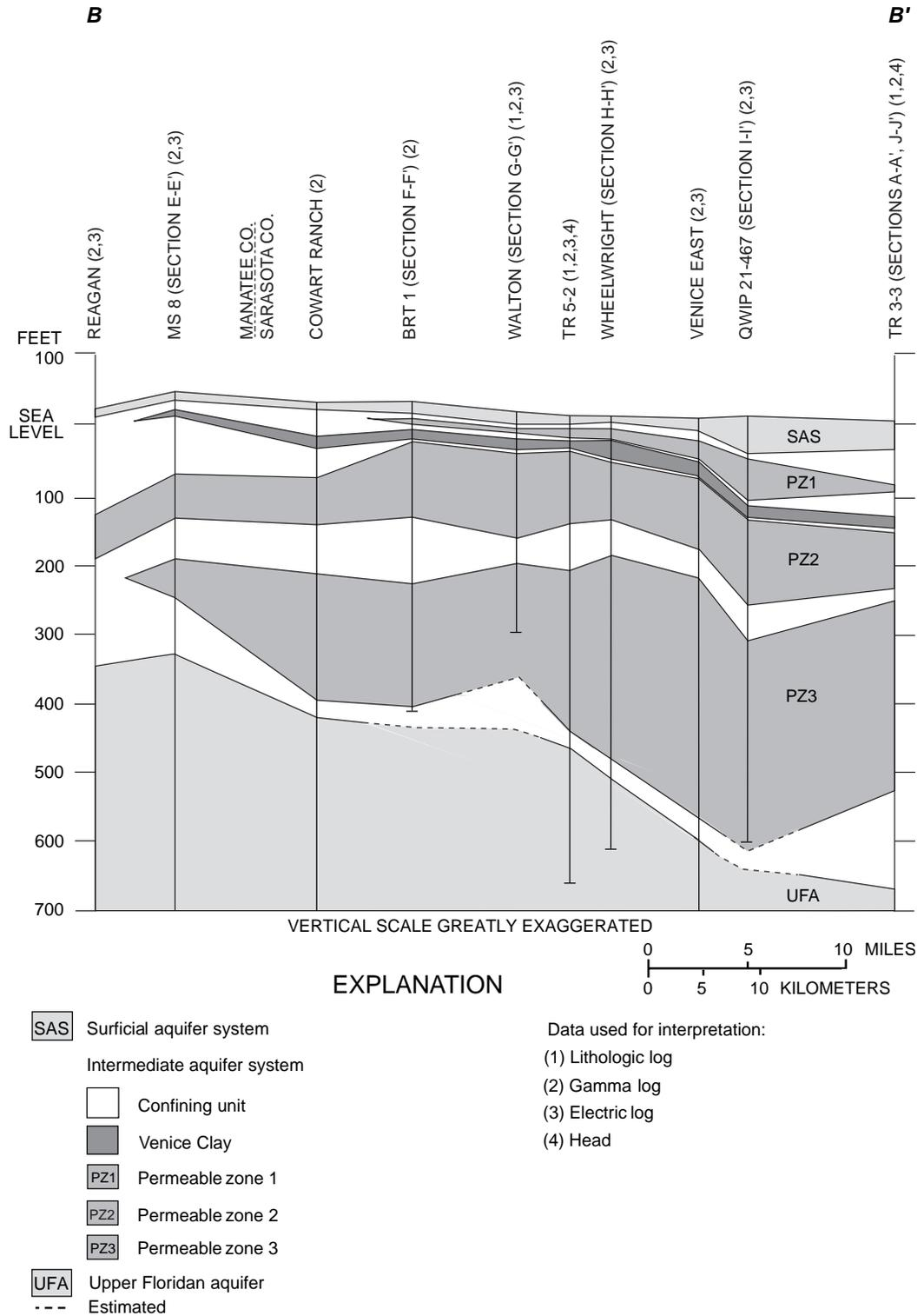
**Figure 8.** Hydrogeologic section B-B' in southwest Florida. (Line of section is shown in figure 6.)
