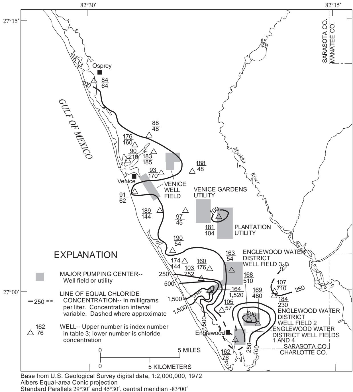
**Figure 29.** Chloride concentration in water from wells open to the intermediate aquifer system, permeable zone 1, in southwest Sarasota County.
