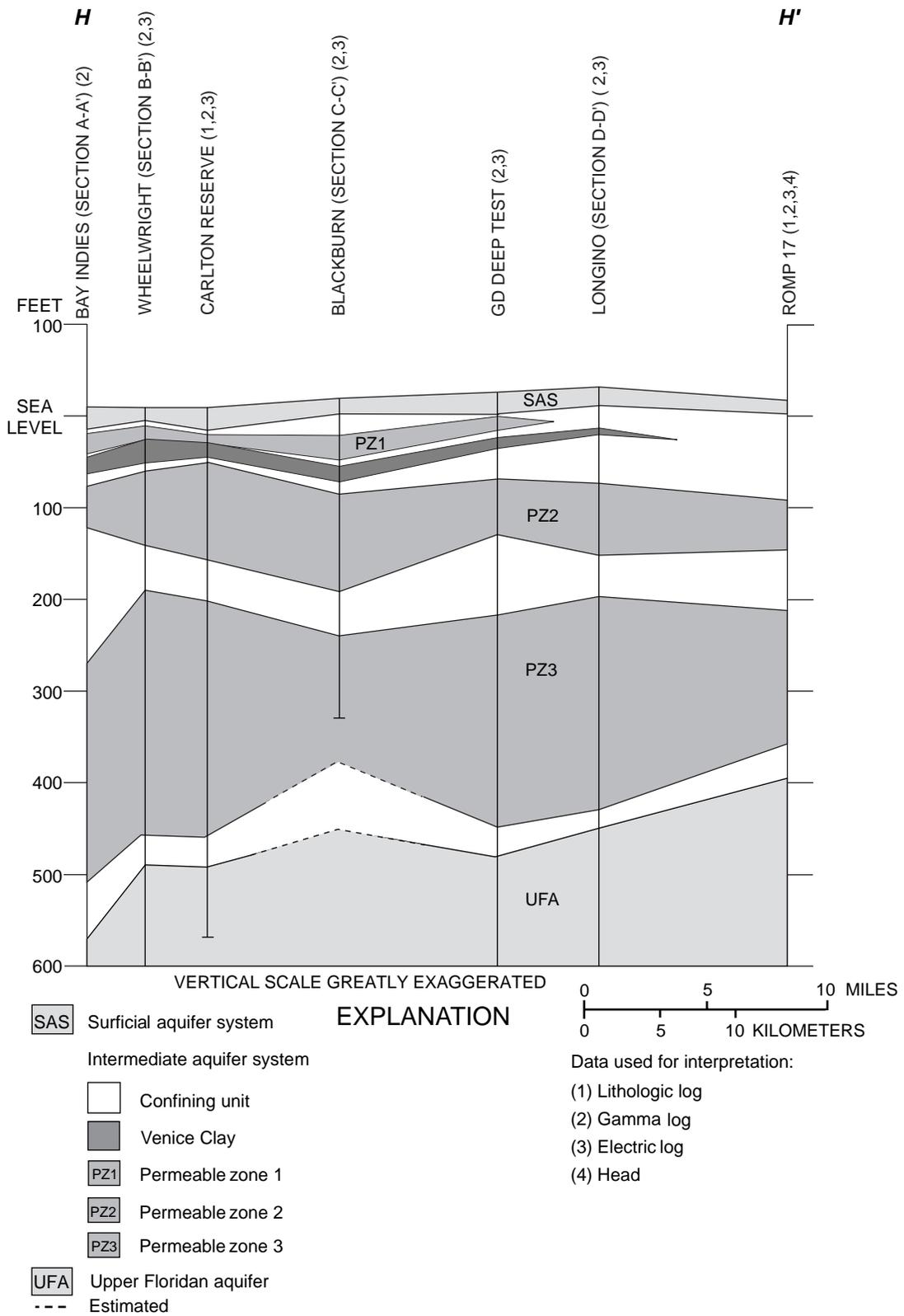
**Figure 14.** Hydrogeologic section H-H' in southwest Florida. (Line of section is shown in figure 6.)
