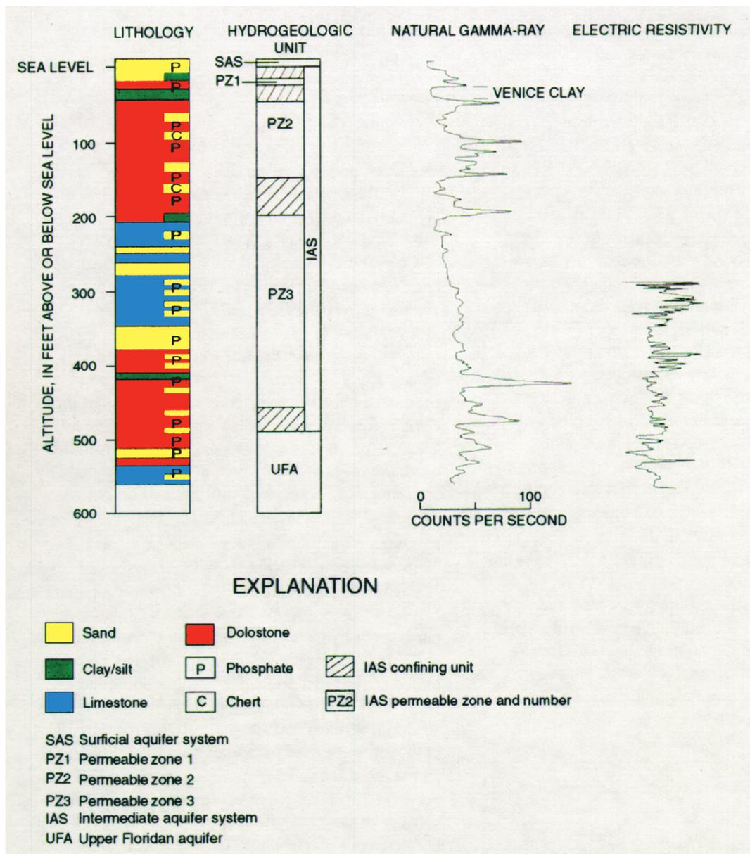
**Figure 2.** Lithologic, hydrogeologic, and geophysical data at the Carlton Reserve test well.
