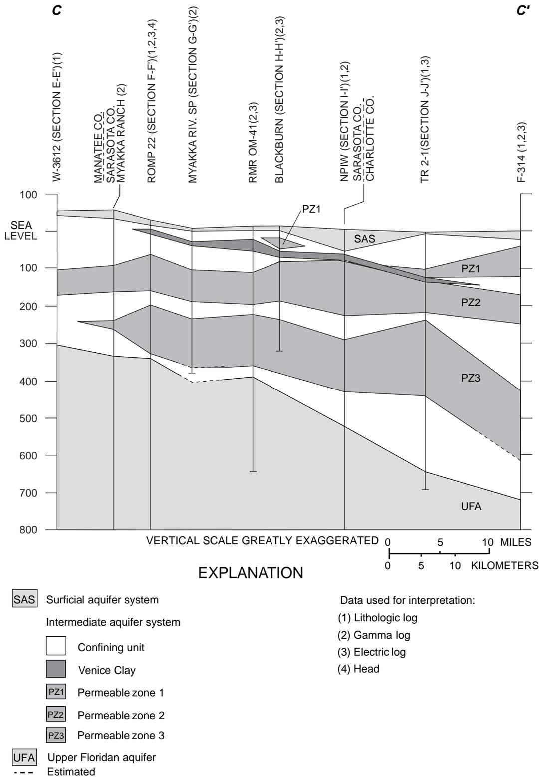
**Figure 9.** Hydrogeologic section C-C' in southwest Florida. (Line of section is shown in figure 6.)
