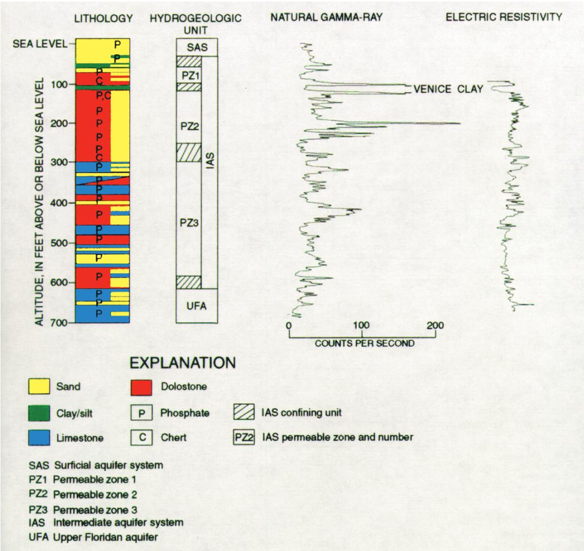
Figure 3. Lithologic, hydrogeologic, and geophysical data at the South Venice test well.
