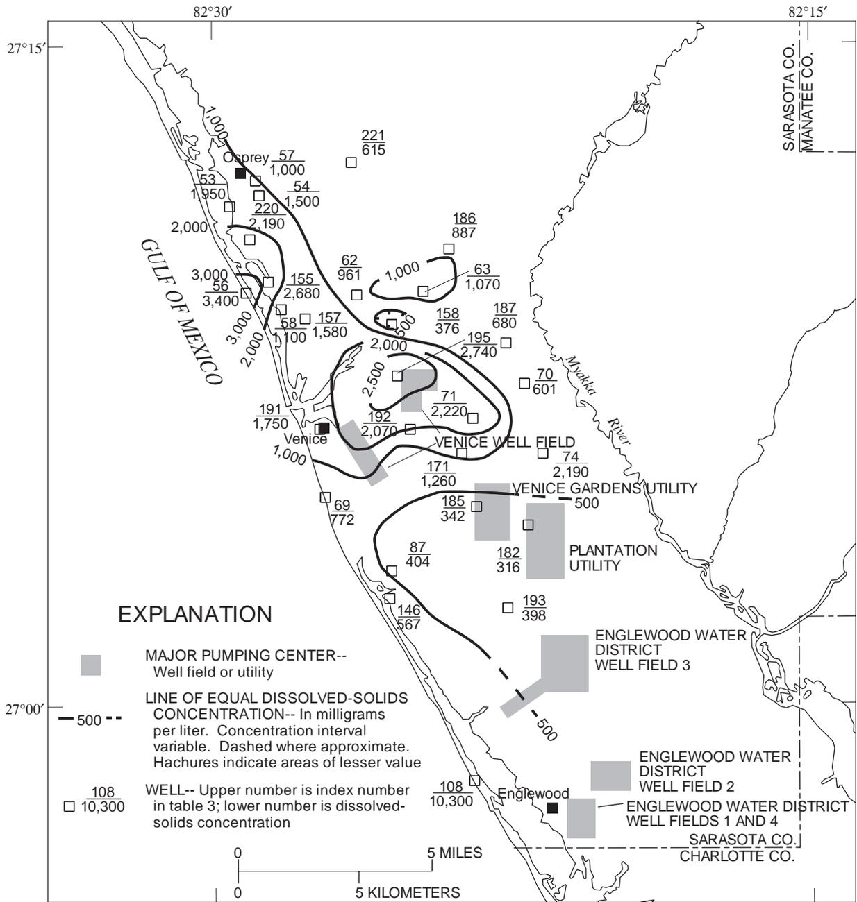
**Figure 35.** Dissolved-solids concentration in water from wells open to the intermediate aquifer system, permeable zone 2, in southwest Sarasota County.
