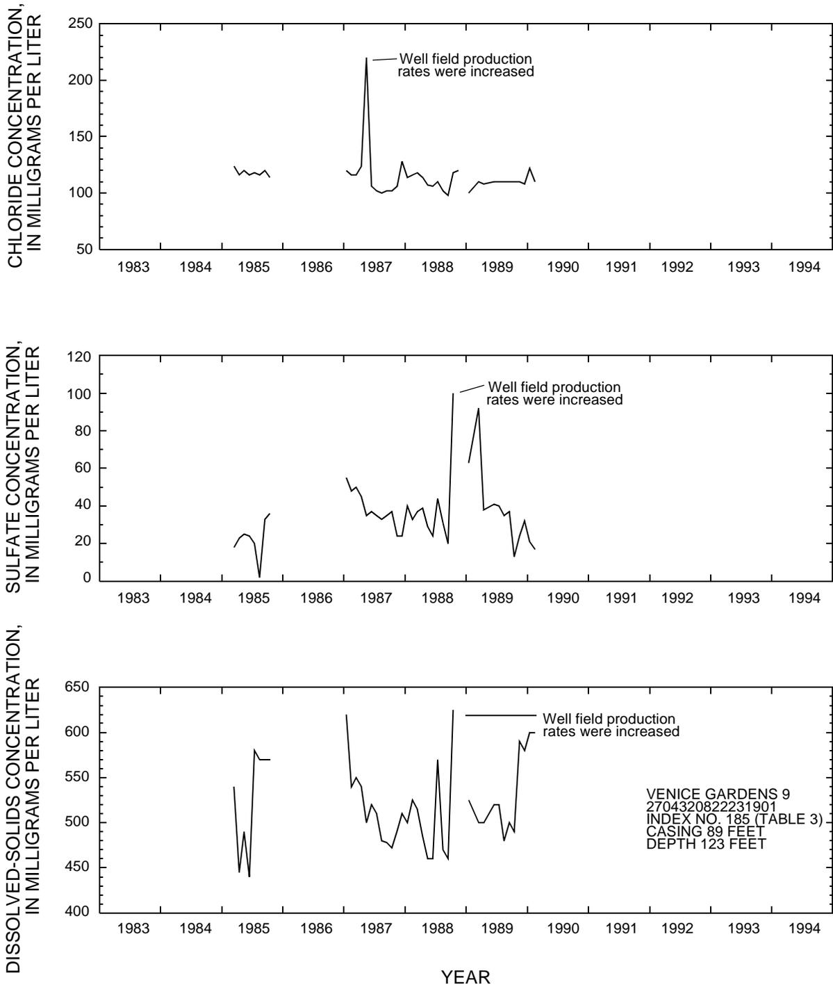
**Figure 42.** Chloride, sulfate, and dissolved-solids concentrations in water from intermediate aquifer system, permeable zone 2, at the Venice Gardens well field monitor well 9, 1985-90. (Data collected by Venice Gardens personnel.)
