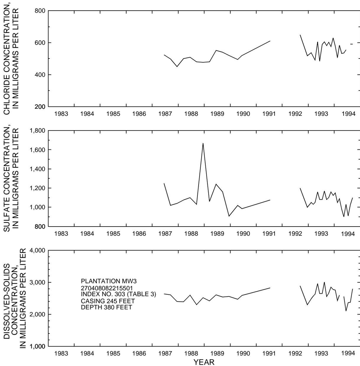
**Figure 46.** Chloride, sulfate, and dissolved-solids concentrations in water from intermediate aquifer system, permeable zone 3, at the Plantation monitor well MW3, 1987-94. (Data collected by Plantation personnel.)
