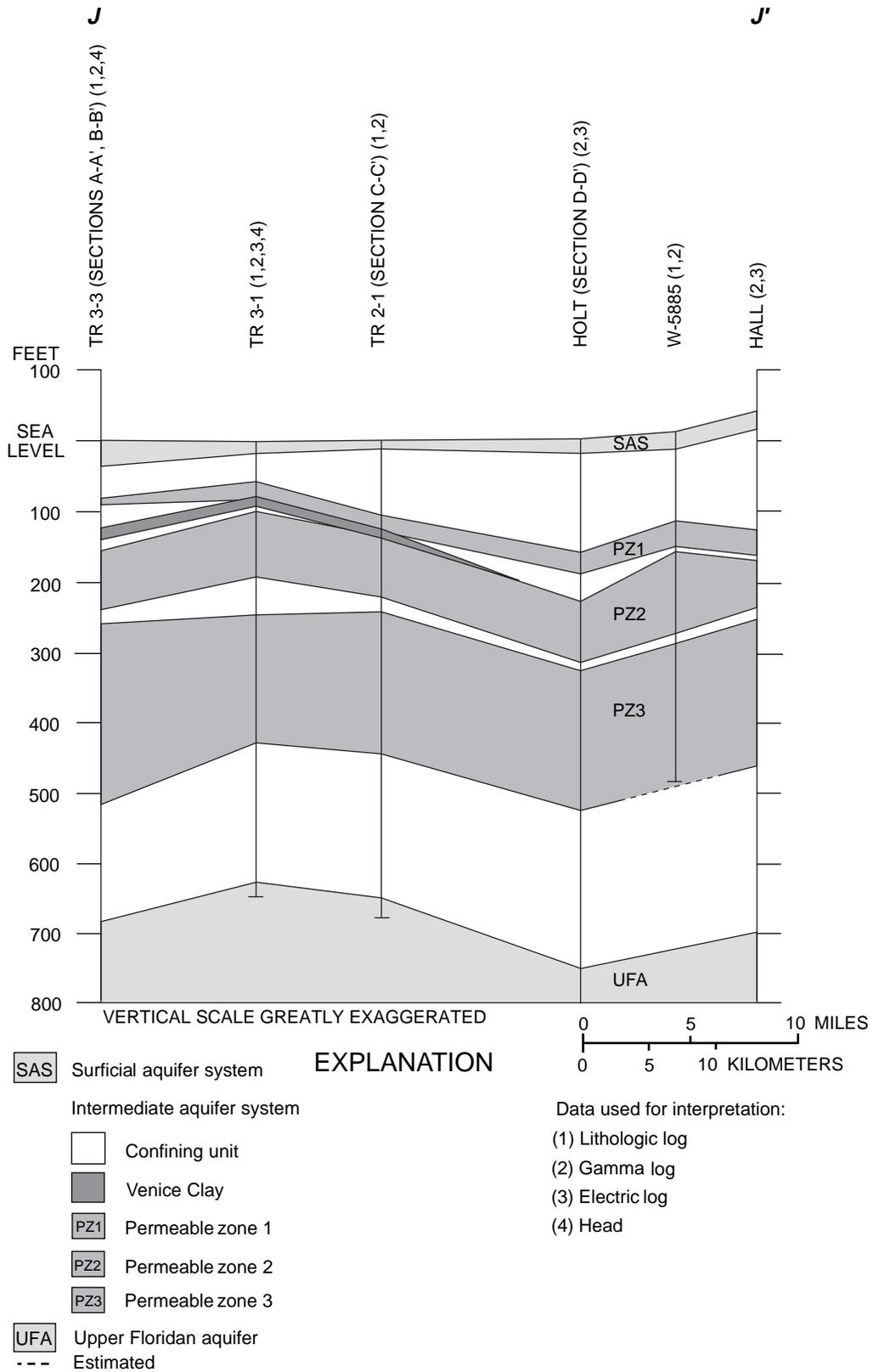
**Figure 16.** Hydrogeologic section J-J' in southwest Florida. (Line of section is shown in figure 6.)
