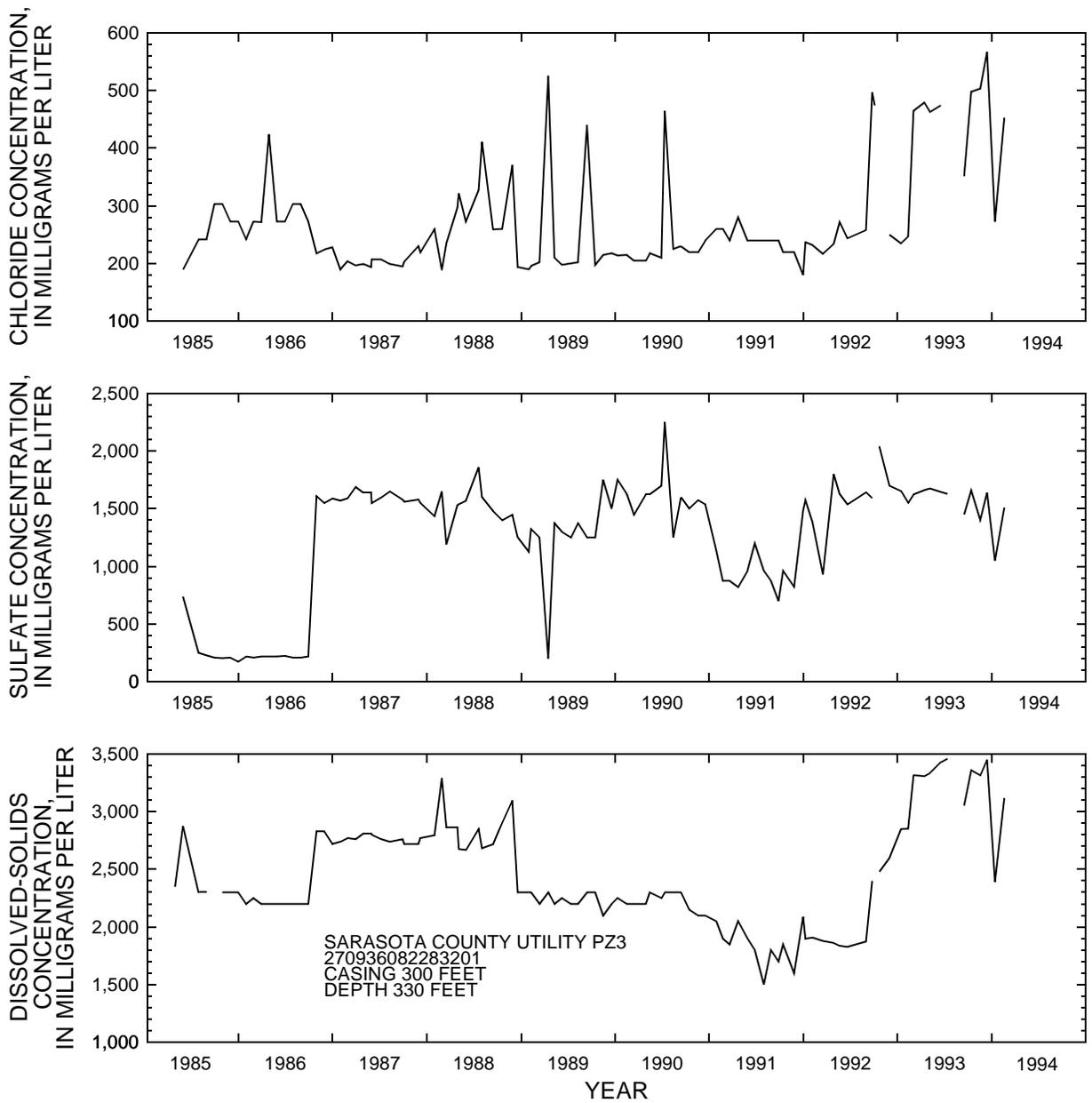
**Figure 47.** Chloride, sulfate, and dissolved-solids concentrations in water from intermediate aquifer system, permeable zone 3, at the Sarasota County Utility well PZ3, 1985-94. (Data collected by Sarasota County personnel.)
