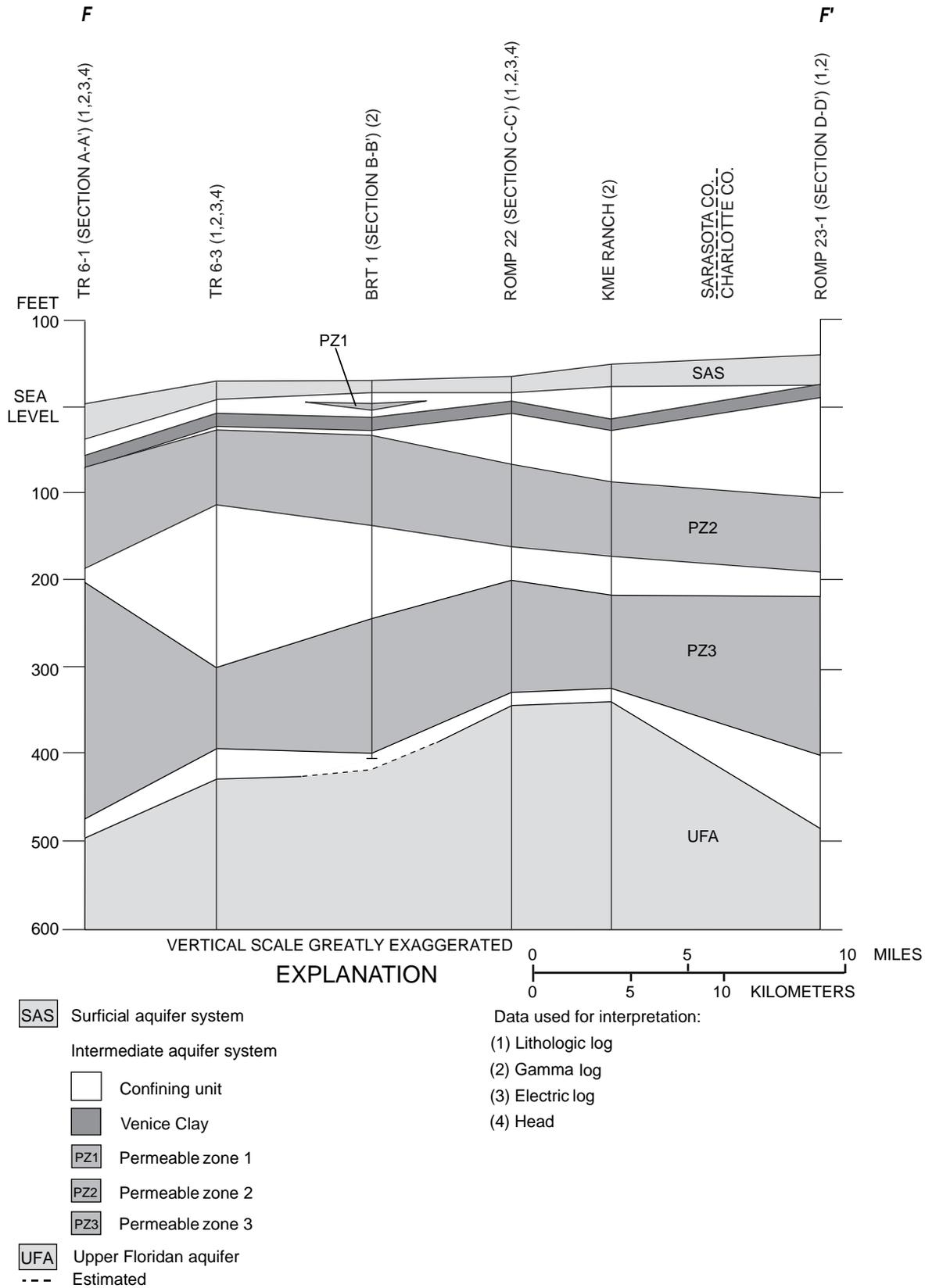
**Figure 12.** Hydrogeologic section F-F' in southwest Florida. (Line of section is shown in figure 6.)
