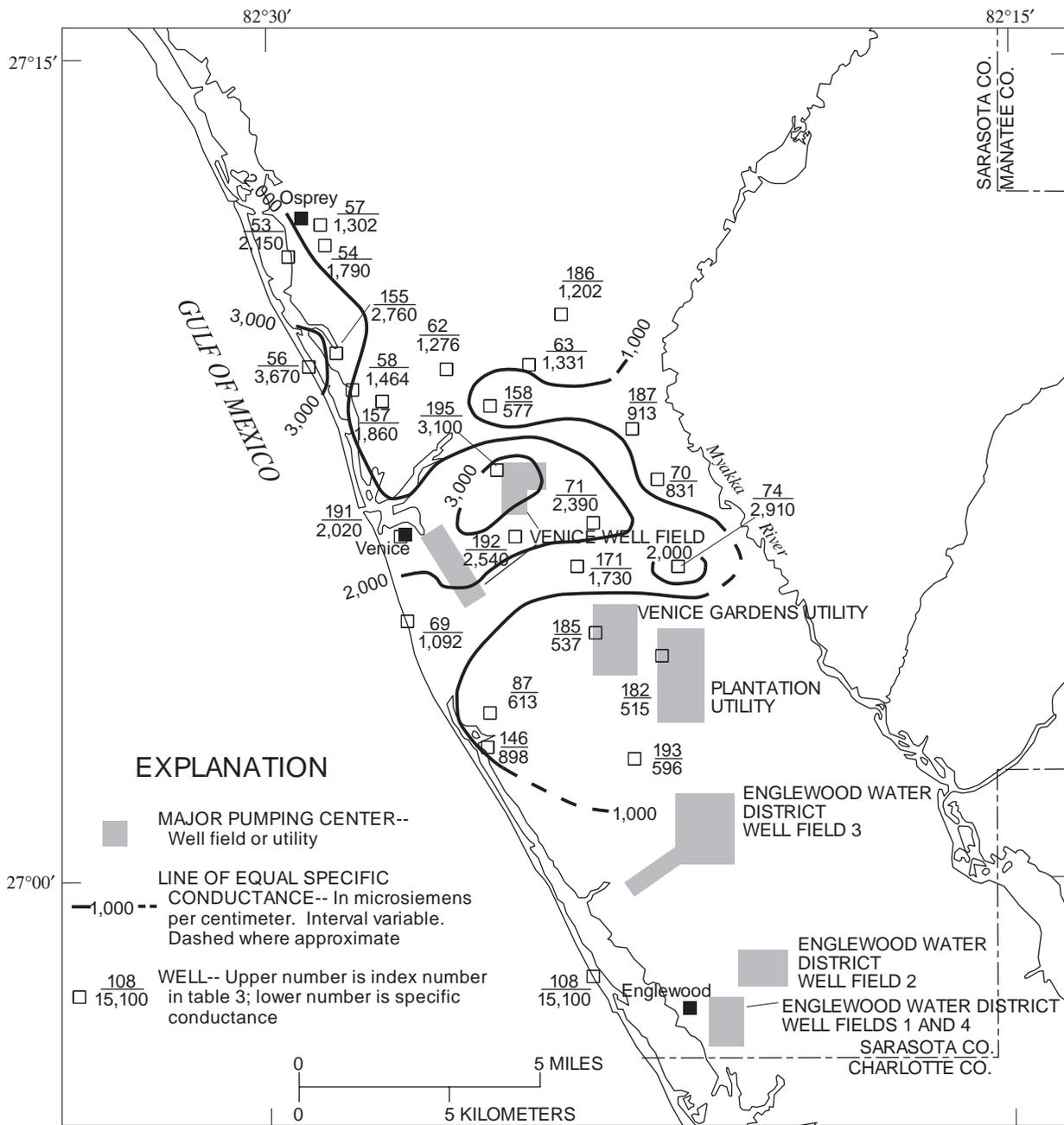
**Figure 36.** Specific conductance of water from wells open to the intermediate aquifer system, permeable zone 2, in southwest Sarasota County.
