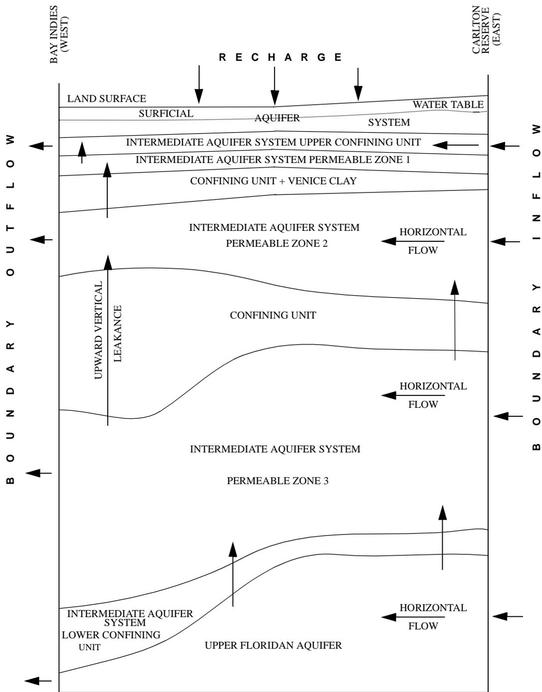
**Figure 53.** Two-dimensional conceptual model of the intermediate aquifer system, southwest Sarasota County. (The section is part of hydrogeologic section H-H', figure 14, from the Bay Indies well to the Carlton Reserve test well.)
