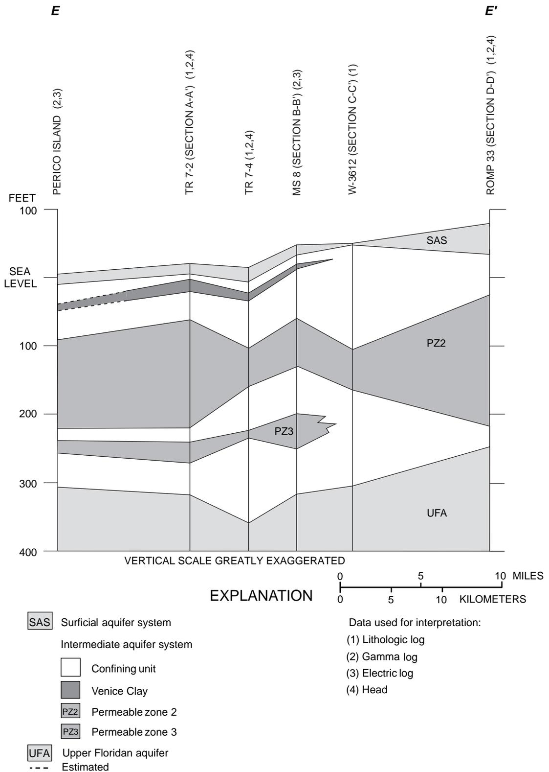
**Figure 11.** Hydrogeologic section E-E' in southwest Florida. (Line of section is shown in figure 6.)
