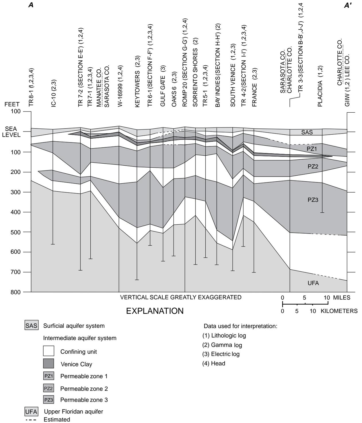
**Figure 7.** Hydrogeologic section A-A' in southwest Florida. (Line of section is shown in figure 6.)
