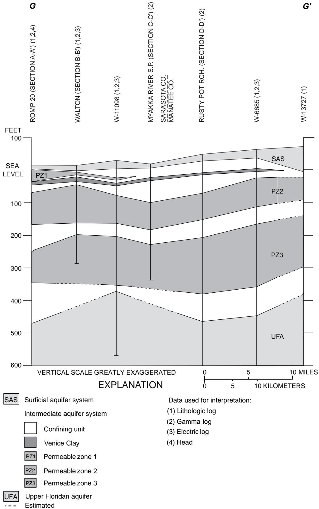
**Figure 13.** Hydrogeologic section G-G' in southwest Florida. (Line of section is shown in figure 6.)
