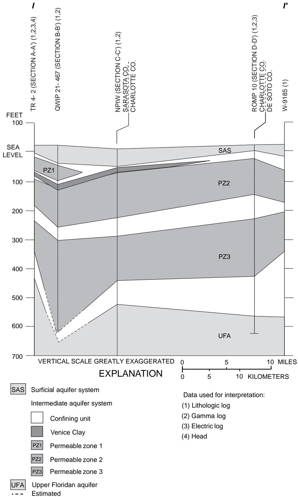
**Figure 15.** Hydrogeologic section I-I' in southwest Florida. (Line of section is shown in figure 6.)
