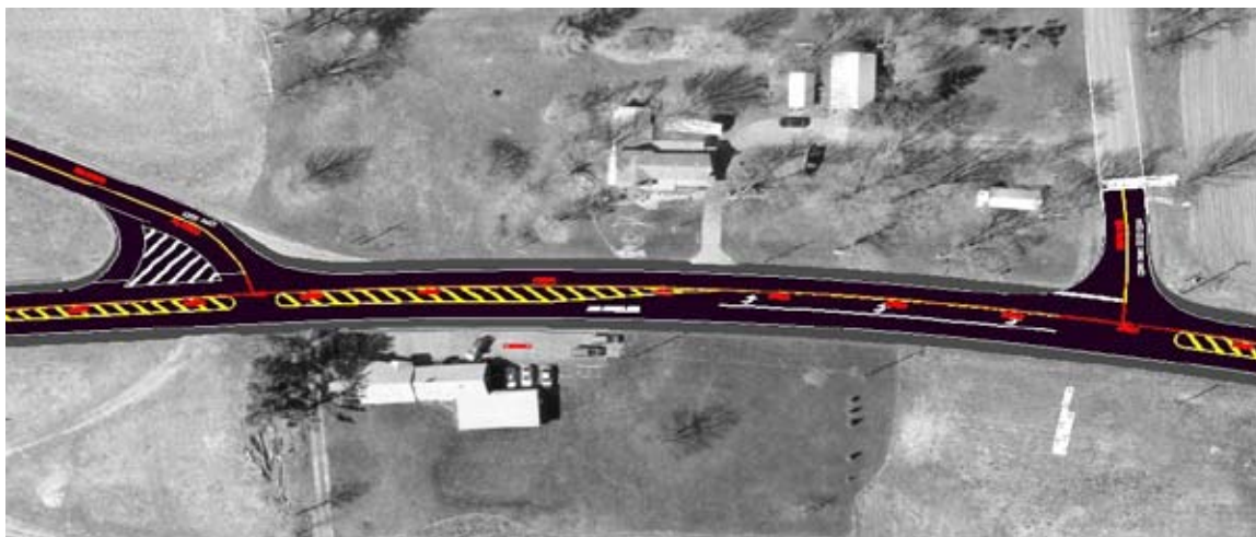
Figure 28. Realignment of intersecting roadways (reduce/eliminate skew) in New York. (Source: Courtesy of NYSDOT)
